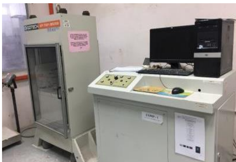
Fig. 2. Universal Testing Machine (GTECH GT-7001-BS300)
