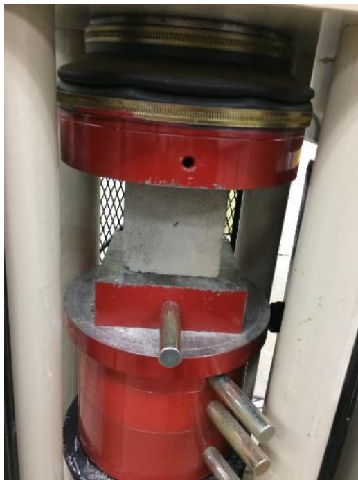
Fig. 3. Axial compressive strength test setup
