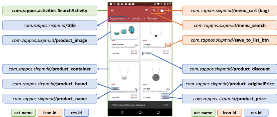
Fig. 3 Multiple GUI text segments (activity name, icon and resource identifiers) that are extracted and preprocessed for NL-based GUI retrieval
