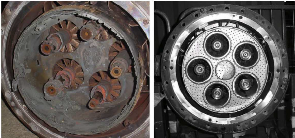
Figure 1.6: Burner assembly damaged by combustion instability (left) and new burner assembly (right) [67]
