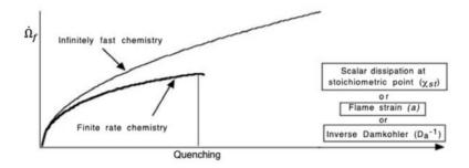
Figure 3-7: Integrated reaction rate as a function of strain in diffusion flames. From [105].
