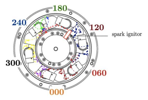
Figure 8-42: Leading point trajectory for case  $\alpha=0^\circ$  and  $\phi=0.7$ . Each point represents a 0.5 ms increment. Different colors were introduced to facilitate the understanding of the trajectory and go in this order: red, blue, green, yellow, purple, brown and navy (The arrows usually serve to follow the change of color). The hollow dots represent the location where the flame reaches the recirculation zone of each injector and manages each injector's ignition
