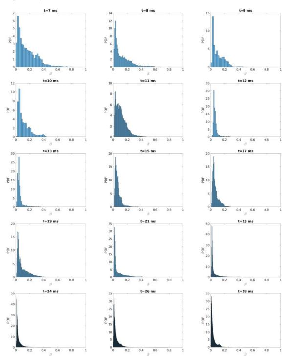
Figure A-7: Evolution of  $\beta$  PDF for an isosurface of q=0.5, Case C ( $p_{ini}=0.5bar$ ,  $t_{delay}=30ms$ ) for various times after spark
