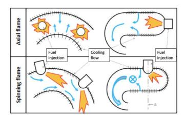
Figure 1-1: Spinning combustion technology (SCT) adapted from [121]
