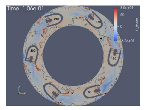
Figure 8-47: Planar cut at the swirler axis for case  $\alpha = 0^{\circ}$  and  $\phi = 0.7$  at t=106 ms showing the tangential velocity (m/s) and a heat release contour at 1e6  $W/m^3$ . Injector location marked with numbers and igniter with the black dot.
