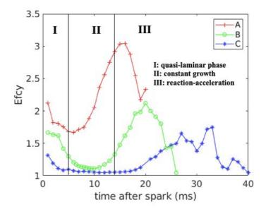
Figure 6-36: Temporal evolution of the average value of efficiency in  $c=0.65\pm0.15$  for the three cases
