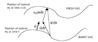
Figure 3-2: Flame speed definitions from [105]
