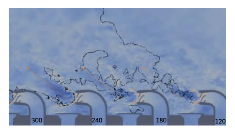
Figure 8-35: Planar projection of annular cut at r=85 mm for case  $\alpha = 23^{\circ}$  and  $\phi = 0.7$  at t=26 ms after igniter start showing the tangential velocity (m/s) and a heat release contour at 1e6  $W/m^3$ . The burnt gases trajectory is indicated by arrows
