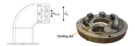
Figure 8-2: (Left) Detailed view of an injector ( $d_e = 19 \text{ mm}$ ,  $d_{hub} = 7 \text{ mm}$ ). (Right) Arrangement in NTNU SCT bench. The cooling slots did not provide any outflow during the ignition experiments to improve repeatability
