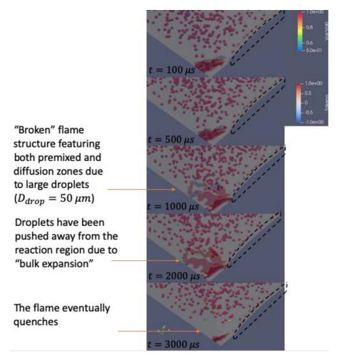
Figure 7-9: Flame evolution colored by Takeno and droplets colored by volume evaporated for case 4 (Failed ignition) ( $\phi_q$ =0  $\phi_l$ =10  $D_{droplet}$ =50  $\mu m$ )
