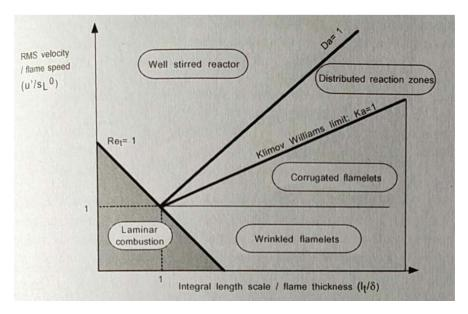
Figure 3-4: Combustion diagram for premixed turbulent combustion from [105]
