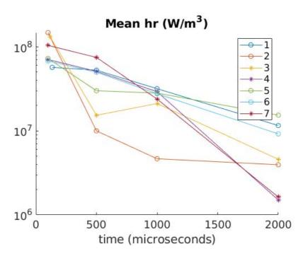
Figure 7-18: Heat release evolution with time. The cases with circles indicate successful flame propagation. The asterisks indicate failed flame propagation
