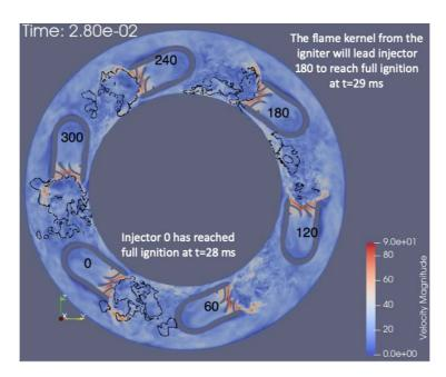
Figure 8-34: Planar cut at swirler axis for case  $\alpha = 23^{\circ}$  and  $\phi = 0.7$  at t=28 ms after igniter start showing the velocity magnitude (m/s) and a heat release contour at 1e6  $W/m^3$ .
