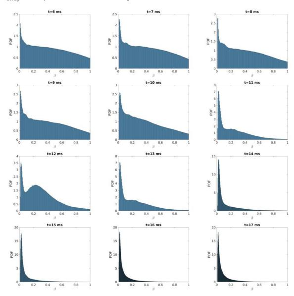
Figure A-6: Evolution of  $\beta$  PDF for an isosurface of q=0.5, Case B ( $p_{ini}=0.5bar$ ,  $t_{delay}=5ms$ ) for various times after spark
