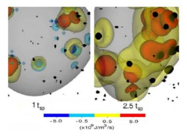
Figure 2-2: Isosurface of heat release (colors) and isosurface of T=1400K (in grey) of a DNS of a monodisperse spray of droplets in homogeneous isotropic turbulence. Left images shows the formation of flame around droplets. Right image shows its merging in a wrinkled flame [96]
