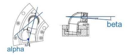
Figure 8-3: Angle definition for NTNU SCT injectors.  $\beta$  fixed to 0 in this study. Two settings for  $\alpha$ : 0 (pointing towards outer wall) and 23 degrees (outlet closer to inner wall)
