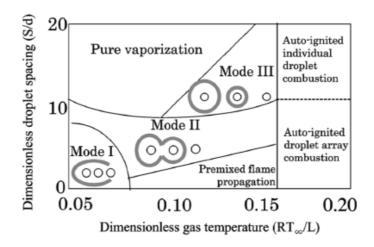
Figure 3-10: Different modes of inter-droplet flame propagation [132]
