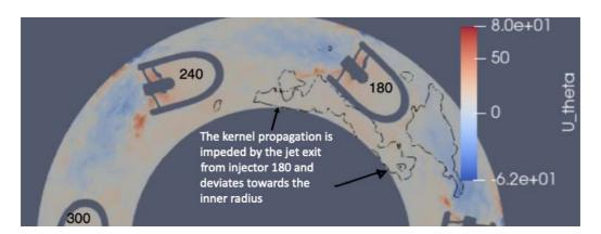
Figure 8-43: Planar cut at the swirler axis for case  $\alpha = 0^{\circ}$  and  $\phi = 0.7$  at t=47.4 ms showing the tangential velocity (m/s) and a heat release contour at 1e6  $W/m^3$ . Injector location marked with numbers and igniter with an arrow.
