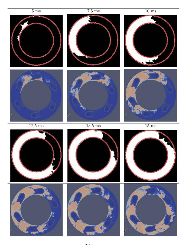
Figure 8-19: Comparison of experimental edge-detection images with temperature fields at plane  $x=1.16D_{inj}$  (parallel to backplane) for case 231 ( $\alpha=23^\circ,\,\phi=1$ ) at various times after spark.
