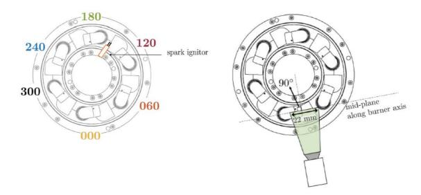
Figure 8-4: Left: Igniter position for NTNU SCT marked in orange and injector position nomenclature, Right: representation of the field of view for each injector (courtesy of Yi-Hao Kwah(NTNU))
