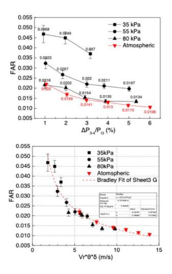
Figure 2-16: Burner ignition boundary line indicated by minimum fuel-air ratio (region above line permits burner ignition) depending on pressure loss across combustor  $\Delta P$  and lining velocity  $v_r$  at different operating pressure. The bottom figure uses the non-dimensional temperature  $\theta = T/(288 \ K)$  and pressure  $\delta = p/(1 \ bar)$  [86]
