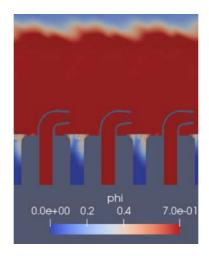
Figure 8-31: Meridional view of the equivalence ratio at the igniter start of the first successful ignition (chamber filled with fuel for 180 ms) for case 237 ( $\alpha = 23^{\circ}$  and  $\phi = 0.7$ )
