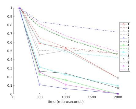
Figure 7-16: Temporal evolution of heat release (solid line) and mass evaporation terms (dashed line). Each variable for each case is made non-dimensional with the value at  $t=100~\mu s$
