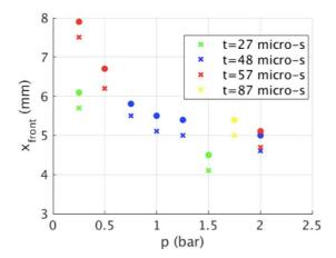
Figure 6-17: Comparison of kernel penetration between the baseline values (h=1.9 mm) (crosses) and an augmented distance over the igniter (h=2.5 mm) (circles) for different initial pressure conditions and at different instants after spark. Radius of the deposit is constant equal to the baseline value (r=2.3 mm)
