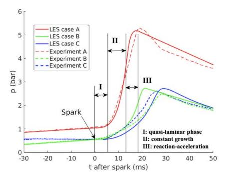
Figure 6-31: Temporal evolution of pressure for cases A ( $p_{ini} = 1$  bar,  $t_{delay} = 5$  ms), B ( $p_{ini} = 0.5$  bar,  $t_{delay} = 5$  ms) and C ( $p_{ini} = 0.5$  bar,  $t_{delay} = 30$  ms). The evolution in all cases can be divided in three phases: a) weak turbulence interaction b) constant flame growth c) burning rate acceleration
