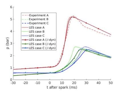
Figure 6-38: Left: Pressure time evolution for the three cases obtained with the staic and the dynamic efficiency formulations and compared to experiments
