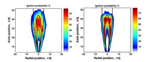
Figure 2-8: Ignition probability map with contours of flammability limits, the black line indicates unity equivalence ratio, showing correspondence of high success rate with stoichiometric conditions [10]
