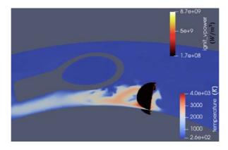
Figure 8-10: View of the semispheric hollow region adopted as a representative location of the energy channel from the igniter and a planar cut of the annular chamber showing that the fluid which as traversed through the deposition zone acquires a temperature of approximately  $3000~\rm K$
