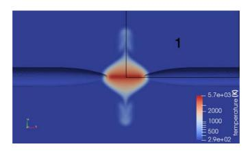
Figure 7-5: View of contours of temperature for the DNS of pin-pin  $\mu s$  after the breakdown. The black rectangle indicates the sector of the domain that will be used as a base for the display of results
