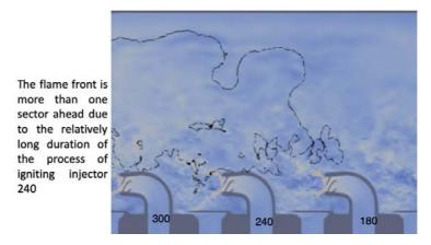
Figure 8-33: Planar projection of annular cut at r=85 mm for case  $\alpha=23^{\circ}$  and  $\phi=0.7$  at t=20 ms after igniter start showing the tangential velocity (m/s) and a heat release contour at 1e6  $W/m^3$ .
