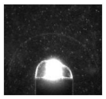
Figure 1-4: Surface discharge a few instants after start [20]
