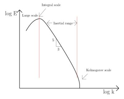
Figure 4-1: Logarithm of the energy vs logarithm of the wave number  $(k = 2\pi/l)$  showing low wave number structures (big scales) having the highest energy. After the integral scale is attained, the logarithm of energy decays at a constant rate until the dissipation scales where energy rapidly decays
