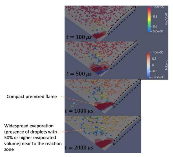
Figure 7-6: Flame evolution colored by Takeno and droplets colored by volume evaporated for case 1 ( $\phi_g$ =0.5  $\phi_l$ =0.125  $D_{droplet}$ =15  $\mu m$ ). The hollow space on the right part of image corresponds to the igniter and there is symmetry with respect to the three planes (left, right and bottom)
