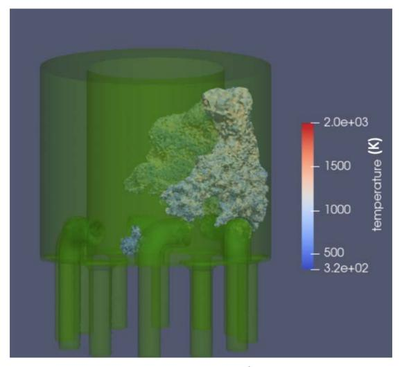
Figure 8-52: Isosurface of heat release at 5e6  $W/m^3$  for case  $\alpha=23^\circ$  and  $\phi=0.7$  (Case 237). As for the case 231, the surface of the consuming reactants covers three injectors while the burnt gases have not arrived to the outlet yet highlighting the difference between terms A and B in the absolute velocity contribution analysis.
