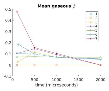
Figure 7-20: Mean  $\phi_g$  inside the reaction region ( $c = 0.65 \pm 0.15$ ). The circles indicate successful flame propagation, asterisks unsuccessful
