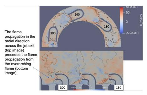
Figure 8-22: (Top) Planar cut at injector showing tangential velocity field (m/s) for case  $\alpha = 23^{\circ}$  and  $\phi = 1$  at t=8.3 ms with a contour of heat release at 5e6  $W/m^3$ . (Bottom) Projection of annular cut at r=85 mm (mid-radius location).
