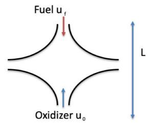
Figure 3-6: Example of a 1D steady diffusion flame
