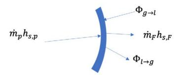
Figure 5-2: Energy balance across the droplet surface
