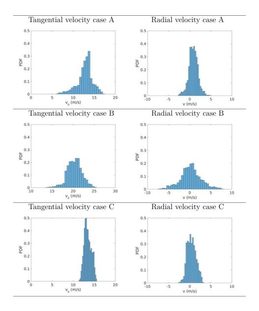
Figure 6-27: Comparison of PDFs of tangential and radial velocities in a sphere of R=3.5cm around the igniter location at the time of spark for the three cases
