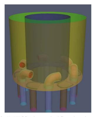
Figure 8-7: Mesh for NTNU SCT showing the different boundaries in different colors
