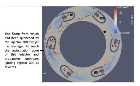
Figure 8-46: Planar cut at the swirler axis for case  $\alpha = 0^{\circ}$  and  $\phi = 0.7$  at t=75.7 ms showing the tangential velocity (m/s) and a heat release contour at 1e6  $W/m^3$ . Injector location marked with numbers and igniter with the black dot.
