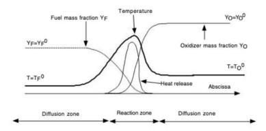
Figure 3-5: Structure of a 1D diffusion flame from [105]
