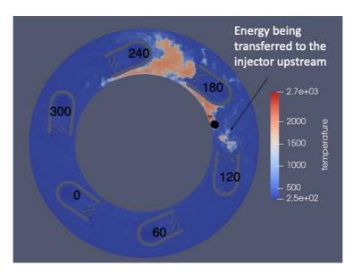
Figure 8-23: Planar cut at injector showing temperature field in Kelvin for case  $\alpha = 23^{\circ}$  and  $\phi = 1$  at t=5.6 ms after igniter start. The location of the igniter is indicated by a black point.
