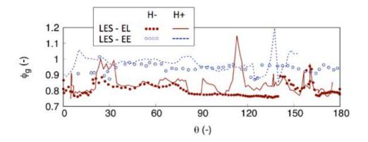
Figure 2-22: Equivalence ratio variation encountered by the leading point showing higher inhomogeneity for the H+ branch (clockwise direction). MICCA spray experiment LES simulations [36]
