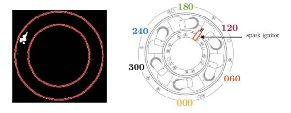
Figure 8-28: First instants of flame propagation in case 237, the first signal of luminescence captured by the camera is near injector 240, indicating the flame kernel has skipped the injector closest to the igniter (180)
