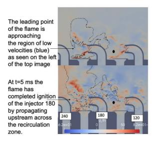
Figure 8-20: Planar projection of annular cut at r=85 mm (mid-radius) for case  $\alpha = 23^{\circ}$  and  $\phi = 1$  at t=4 ms (Top) and t=5 ms (Bottom) after igniter start showing the tangential velocity (m/s) and a heat release contour at 5e6  $W/m^3$ . The injector numbers are indicated in the inlet tubes.
