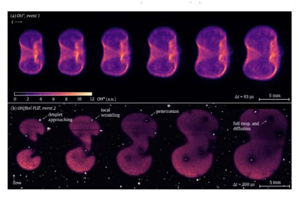
Figure 2-12: (a)  $OH^*$  and (b) OH/fuel PLIF images indicating heat release zones and physical effects for the inter-droplet propagation regime [43]
