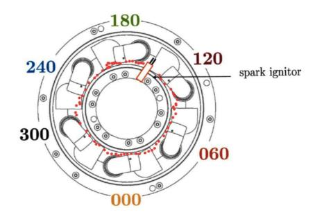
Figure 8-25: Leading point trajectory for case  $\alpha=23^\circ$  and  $\phi=1$  . Each point represents a 0.2 ms increment.
