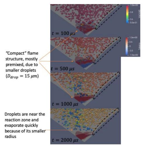
Figure 7-10: Flame evolution colored by Takeno and droplets colored by volume evaporated for case 5 (Successful ignition) ( $\phi_q$ =0  $\phi_l$ =10  $D_{droplet}$ =15  $\mu m$ )
