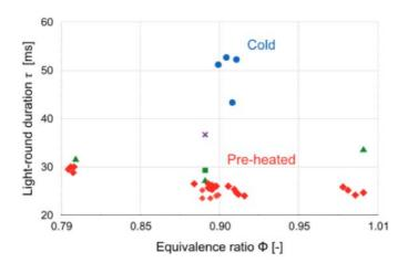
Figure 2-21: Comparison of CFD results to experiments for light around duration in the MICCA experiment. Red diamods are experimental results for the case where walls are preheated, green triangles are CFD results for the same conditions, blue circles are experimental results for the case where walls are at ambient temperature, the purple cross indicates CFD result for that condition.
