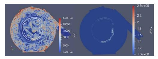
Figure 6-37: Left: Vorticity field with a white contour indicating flame position for case B at t=6ms after spark. Right: Efficiency field showing high values only where wall-originated vorticity is interacting with the flame.
