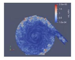
Figure 6-24: Field of  $\nu_{turb}/\nu_{lam}$  after filling up to p=1 bar for case A, before spark
