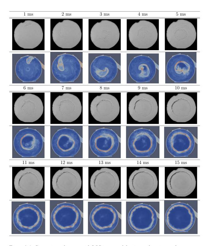
Figure A-2: Comparison of images with LOS integrated density gradient images from LES for case B  $(p_{ini}=0.5bar,\,t_{delay}=5ms)$  at various times after spark. Dynamic efficiency formulation
