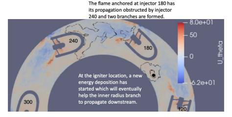
Figure 8-44: Planar cut at the swirler axis for case  $\alpha = 0^{\circ}$  and  $\phi = 0.7$  at t=64.5 ms showing the tangential velocity (m/s) and a heat release contour at 1e6  $W/m^3$ . Injector location marked with numbers and igniter with the black dot.
