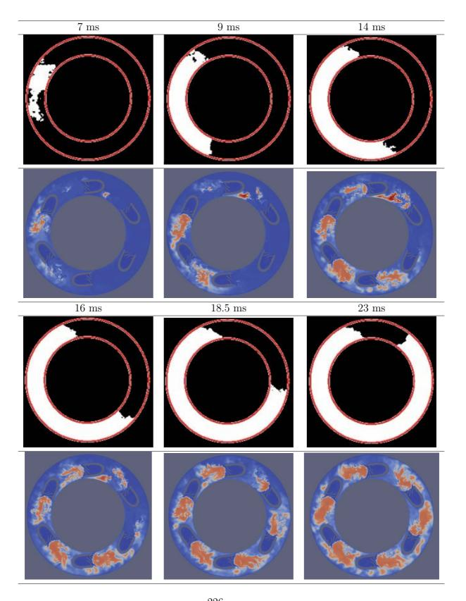
Figure 8-30: Comparison of experimental edge-detection images with temperature fields at plane  $x=1.58D_{inj}$  (parallel to backplane) for case 237 ( $\alpha=23^\circ,\,\phi=0.7$ ) at various times after spark.
