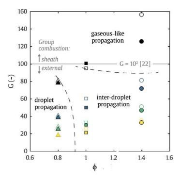
Figure 2-9: Different ignition modes depending on the group combustion number (G) and equivalence ratio for two different fuels (Jet A, hollow points) and a renewable fuel (ATJ-8, filled points) [43]. Black, blue, green and yellow colors correspond to a SMD of 15, 20, 27, 33  $\mu$ m
