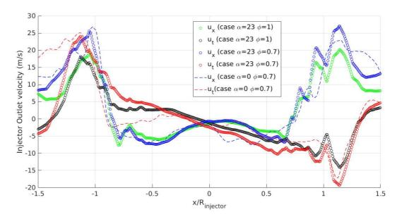
Figure 8-14: Averaged velocity profiles at 2.5 mm  $(0.26 R_{inj})$  downstream the injector face from LES calculations. The axial component is normal to the injector face, while the transversal component is perpendicular to the normal and parallel to the annulus axis
