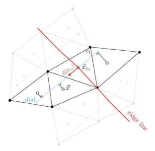
Figure 4-4: Illustration of the application of thickening in a direction normal to the ridge line. The process is the following: The point C1 is detected to be in the flame region. Then, its perpendicular direction and distance to the ridge line is computed. Finally, thickening is applied to the cells whose center are closer than a certain distance "dist". The "dist" parameter is user-defined. From [117]
