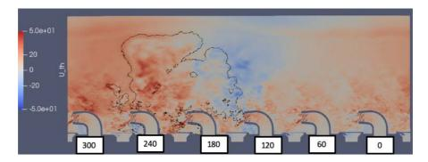
Figure 8-27: . Projection of annular cut at mid-radius for case  $\alpha=23^\circ$  and  $\phi=1$  at t=6 ms showing tangential velocity in m/s. The reddish zone on the right of the image indicates enhanced azimuthal velocity, while the bluish part represents the contrary sense of azimuthal motion
