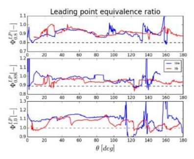
Figure 2-19: Equivalence ratio at the leading point along the azimuth of the rig during ignition (MICCA experiment) showing richer conditions than the ones at the injection point marked by black discontinuous line [68]. H+ indicates the flame branch travelling in clockwise direction and H- the one travelling anticlockwise.
