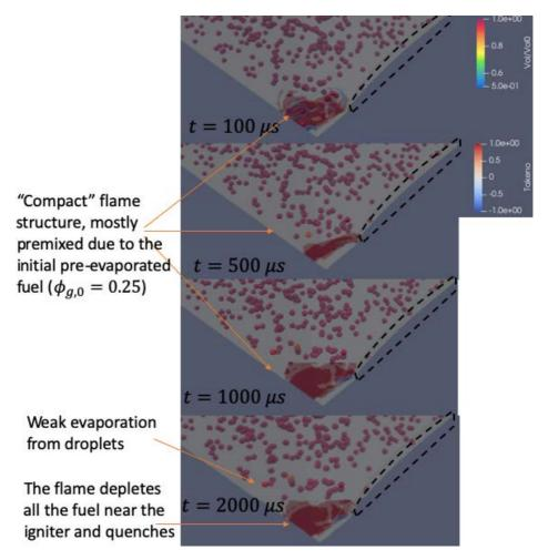
Figure 7-12: Flame evolution colored by Takeno and droplets colored by volume evaporated for case 7 (Failed ignition) ( $\phi_q$ =0.25  $\phi_l$ =10  $D_{droplet}$ =50  $\mu m$ )
