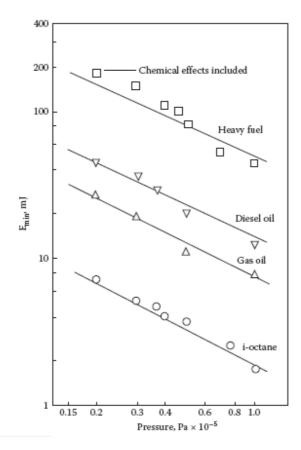
Figure 2-5: MIE dependence with pressure for mean flow velocity=15 m/s,  $\phi$ =0.65, SMD=60 $\mu$ m showing fair agreement for experiments and the analytical formula in Eqs. 2.1 and 2.4 [17]
