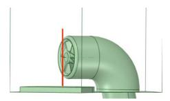
Figure 8-15: Station where velocity profiles are measured (2.5 mm (0.26  $R_{inj}$ ) down-stream the injector face). The axial component is normal to the injector face, while the transversal component is perpendicular to the normal and parallel to the annulus axis
