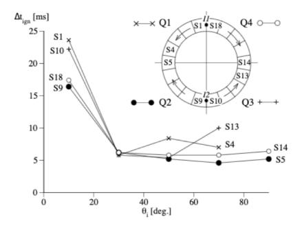
Figure 2-25: Ignition time variation showing that anticlockwise sectors (e.g. 1-4) have higher delays with respect to clockwise (e.g 18-14) [23]
