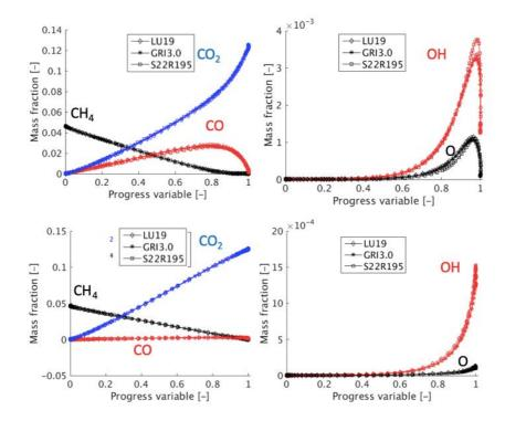
Figure 6-20: Methane-air combustion: comparison of species profiles in a lean premixed flame for inlet conditions of p=1 bar, 320K and  $\phi = 0.83$  at strain rate equal to 2000  $s^{-1}$  (top) and 20000  $s^{-1}$  (bottom) or Lu19, GRI3.0 and S22R195. Progress variable based on  $CH_4$ .
