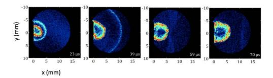
Figure 6-7: Ardiden 3 igniter discharge kernel evolution for P=1 bar and T=293 K. Visualisation from 23  $\mu s$  to 70  $\mu s$ . Positions are reported in mm from the igniter surface, along the symmetry axis.
