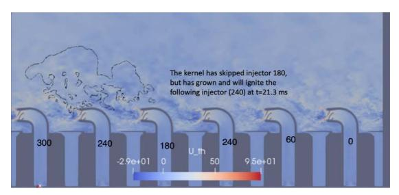
Figure 8-32: Planar projection of annular cut at r=85 mm for case  $\alpha=23^{\circ}$  and  $\phi=0.7$  at t=16 ms after igniter start showing the tangential velocity (m/s) and a heat release contour at 1e6  $W/m^3$ .
