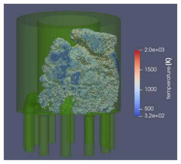
Figure 8-51: Isosurface of heat release at 5e6  $W/m^3$  for case  $\alpha=23^\circ$  and  $\phi=1$  (Case 231). The surface of the consuming reactants covers three injectors while the burnt gases have not arrived to the outlet yet.
