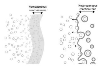
Figure 3-12: "Homogeneous" (Left) and "heterogeneous" combustion modes [98]
