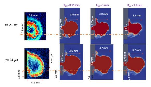
Figure 6-10: (Left) Experimental SBOS images at t=21  $\mu s$  and 24  $\mu s$ . (Right) Temperature contours at 620 K for three values of  $R_{arc}$ . The dotted line indicates the symmetry axis of the igniter.
