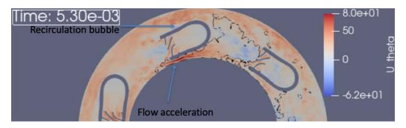
Figure 8-21: Planar cut at injector showing tangential velocity field (m/s) for case  $\alpha = 23^{\circ}$  and  $\phi = 1$  at t=5.3 ms after igniter start with a contour of heat release at 5e6  $W/m^3$  showing flame propagation acceleration.
