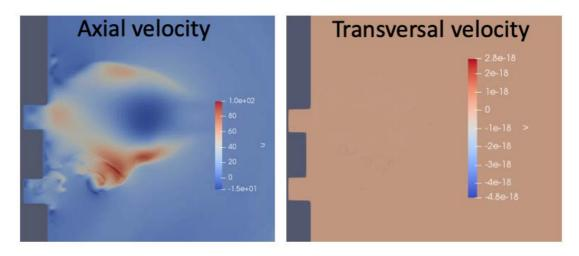
Figure 6-12: Axial and transversal velocity from LES showing the kernel has no transversal movement at t=49  $\mu s$  after spark.  $R_{arc} = 0.75$  mm.
