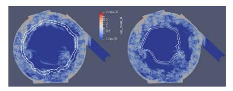
Figure 6-34: Contour fields of  $u'_{\Delta}/S_l$  for case C at t=11 ms after spark for case B (left) and case C (right)
