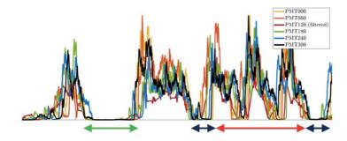
Figure 8-40: Photomultiplier signals for case  $\alpha = 0^{\circ}$  and  $\phi = 0.7$  showing oscillating light-around behavior and arrows indicating dissimilar duration of periods of low chemical activity (Courtesy of Yi-Hao Kwah (NTNU))
