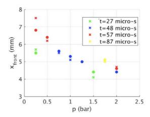
Figure 6-16: Comparison of kernel penetration between the baseline values (r=2.3 mm) (crosses) and a deposit of r=2.8 mm (circles) for different initial pressure conditions and at different instants after spark. Height over igniter is constant equal to the baseline value (h=1.9 mm)
