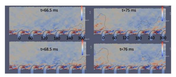
Figure 8-49: . Projection of annular cut at r=85 mm (mid-radius) for case  $\alpha=0^\circ$  and  $\phi=0.7$  showing tangential velocity (m/s). The instants correspond to the ignition of injector 240 (left) and injector 300 (right) and show a weak contribution of the bulk flow expansion for case 07
