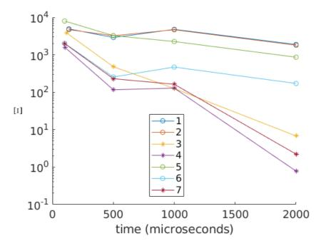
Figure 7-17: Temporal evolution of non-dimensional ratio of heat release by mass evaporation term  $\Xi = hr * V_{flame}/(\dot{m}_{evap} * \Delta H_r)$  Circles mark successful ignition, while asterisks mark failures
