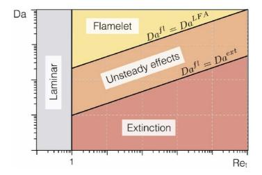
Figure 3-8: Combustion diagram for diffusion turbulent combustion [40]
