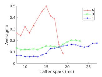
Figure 6-40: Evolution of the volume integral of the wrinkling parameter  $\beta$  over an isovolume of  $c=0.65\pm0.15$ . Each data point is obtained by a spatial average from a instantaneous solution at a period of 1 ms after spark.
