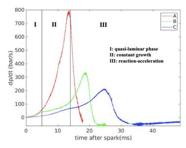
Figure 6-32: Temporal evolution of the change of pressure with time with lines indicating the phase boundaries for cases B and C. For case A, phase II takes place between  $5 < t < 10~\mathrm{ms}$
