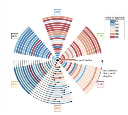
Figure 8-29: Top representation of the light-around of case  $\alpha=23^\circ$  and  $\phi=0.7$  (Courtesy of Yi-Hao Kwah (NTNU)). Each ring consists of one run (There are 20 experiment runs of this case in total)
