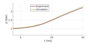
Figure 6-23: Temporal pressure evolution for a case with  $p_{ini}$ =1bar,  $T_{ini}$ =300 K,  $\phi$ =0.7
