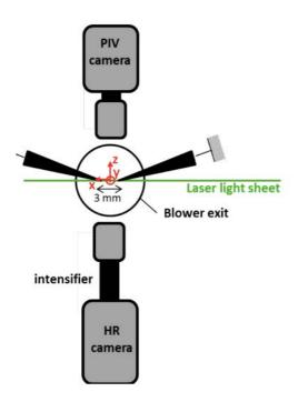
Figure 7-1: CORIA pin-pin experimental setup, adapted from [66]
