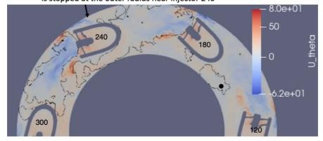
Figure 8-45: Planar cut at the swirler axis for case  $\alpha = 0^{\circ}$  and  $\phi = 0.7$  at t=72.4 ms showing the tangential velocity (m/s) and a heat release contour at 1e6  $W/m^3$ . Injector location marked with numbers and igniter with the black dot.
