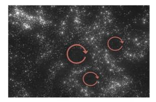
Figure 3-11: Preferential segregation caused by homogeneous isotropic turbulence. Large turbulent structures are marked with an arrow [142]
