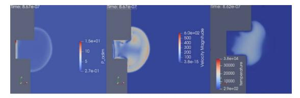
Figure 6-9: Results for  $p^* = p/p_{amb}$ , velocity (m/s) and temperature (K) for the cylindrical ignition approach at t=0.86  $\mu s$  after spark (Transition between breakdown and arc phase)
