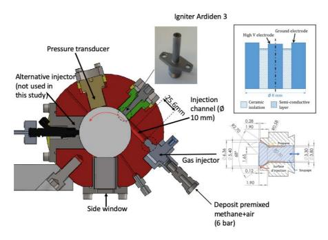
Figure 6-18: Sectional view of the chamber showing injection from the channel on the right, igniter at the top of the cylinder and in anticlockwise order: pressure sensor, liquid injector (not used in this study), window.
