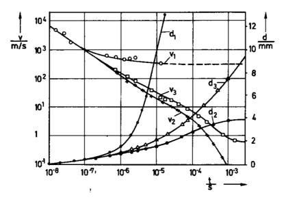
Figure 2-1: Diameters (d) and expansion velocities (v) of the kernel in an ignition experiment from [78] consisting of an automotive pin-pin igniter showing that the kernel expansion is governed by the movement of the shock for t<0.5  $\mu$ s. The indices indicate: 1: shock in air at 1 bar; 2: plasma in air at 1 bar; 3: electrical and chemical plasma respectively in a stoichiometric  $CH_4$ -air mixture at 1 bar
