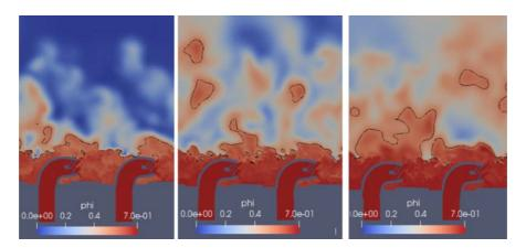
Figure 8-41: Case  $\alpha = 0^{\circ}$  and  $\phi = 0.7$  meridional view of the equivalence ratio with a contour line for  $\phi = 0.52$  (lower flammability limit) after filling for t=62, 80 and 99 ms. The last image coincides with the first successful injector ignition (injector 180)
