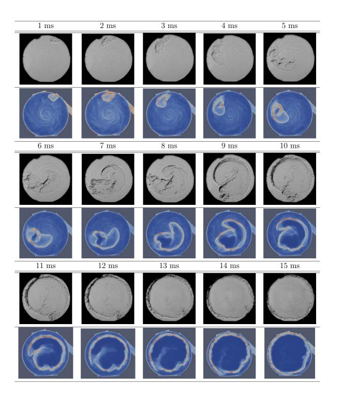
Figure A-1: Comparison of images with LOS integrated density gradient images from LES for case A  $(p_{ini}=1bar,\ t_{delay}=5ms)$  at various times after spark. Dynamic efficiency formulation
