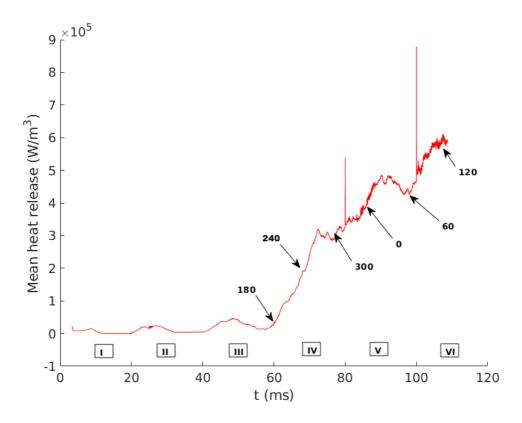
Figure 8-48: Temporal heat release evolution for case  $\alpha=0^\circ$  and  $\phi=0.7$ . The arrows indicate the instant for injector ignition. The time origin coincides with the first sparking from the igniter, which follows a cycle of period 20 ms as marked by the roman numbers along the x-axis. The spikes at t=80 and 100 ms are caused by the igniter spark start of periods V and VI
