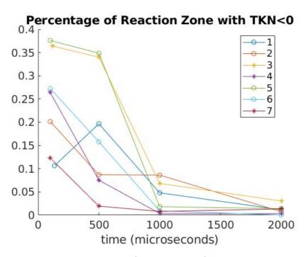
Figure 7-21: Fraction of reaction zone ( $c = 0.65 \pm 0.15$ ) with negative Takeno (indicating diffusion combustion regime). The circles indicate successful flame propagation, asterisks unsuccessful
