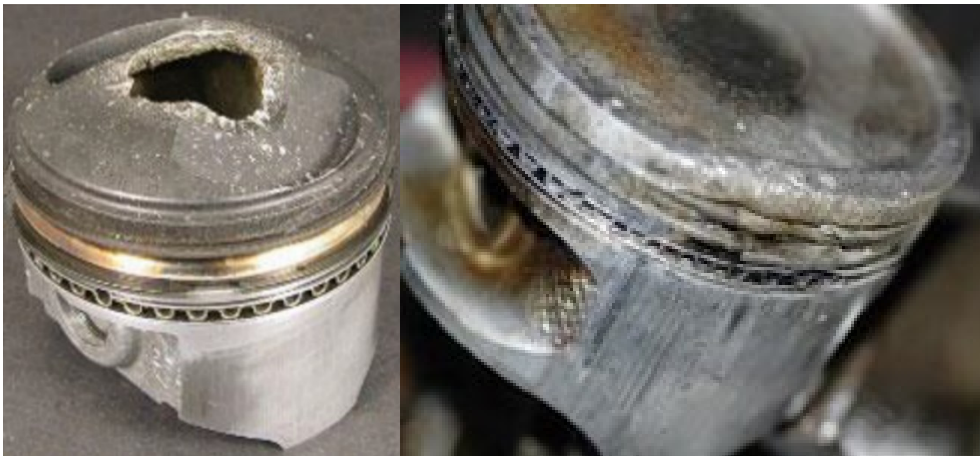
Figure 2-14 Example of engine piston damaged by heavy knock.
