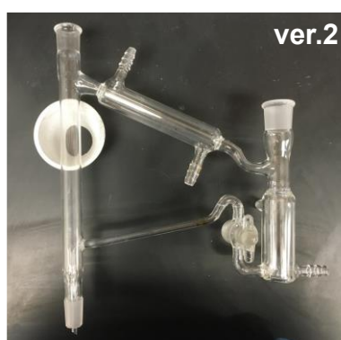
Figure A4. The design plan of the custom glassware and pictures of the modified versions.
