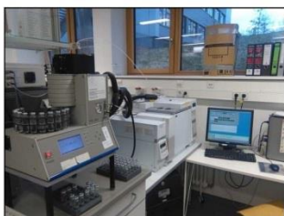
Figure 3: P&T-GC-QMS system was used for the CI-CSIA: Agilent 6890N GC coupled to an Agilent 5973N QMS (Santa Clara, USA) and a P&T system PTA 3000 by IMT (Vohenstrauß, Germany).
