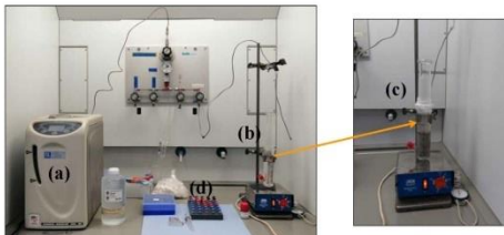
Figure 2: (a) Hydrogen generator (Schmidlin, NMH2 160, Germany) used to saturate the deionized water with hydrogen (b) Reactor with a sampling port near the bottom (c) Close up view of the reactor as the reaction proceeds (d) samples taken
