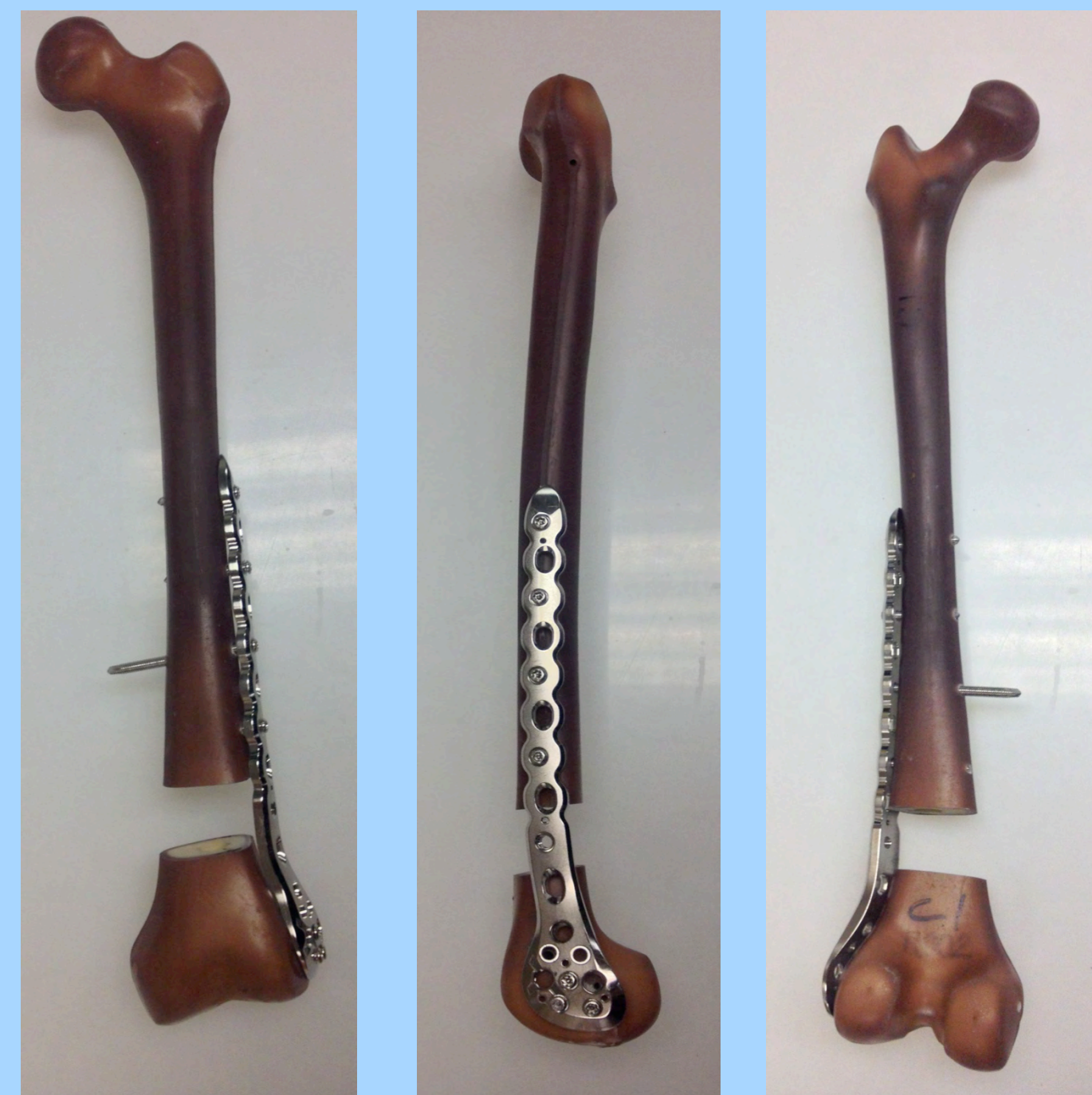
Figure 2. Sawbone femur model with distal femur locking plate and fracture gap (A). AP and oblique x-ray views of distal femur model with 1mm chrome steel bearings visualized as labeled by arrows (B).
