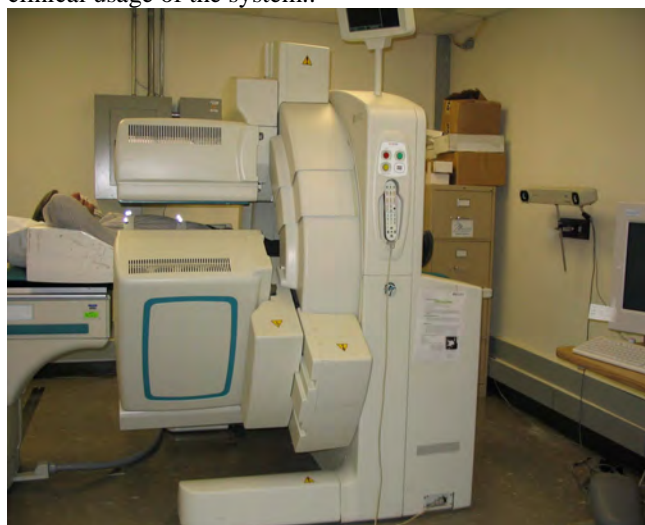
Fig. 1. The Polaris system is seen on the far right mounted on the wall. The white spots on the 2 belts are the attached IR reflecting spheres. Volunteer and SPECT camera setup was performed by a technologist matching what would be employed clinically.
