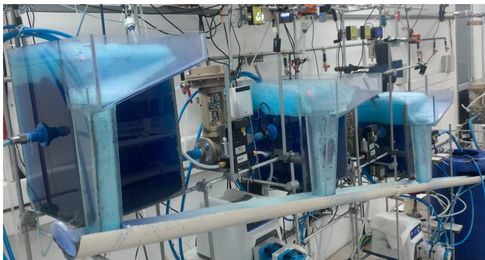
Fig. 3. Experimental system with froth overflowing from the top of each bank.
