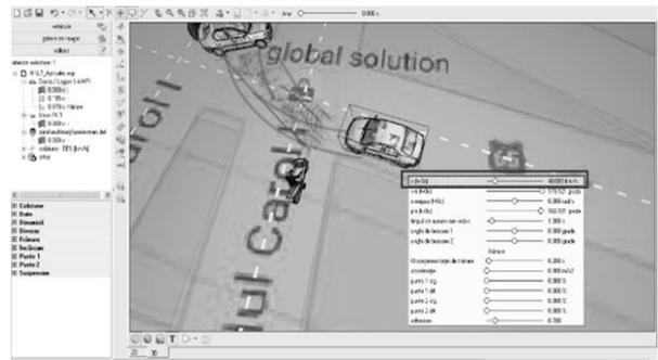
Fig.14 Setting pre-collision vehicle data.
