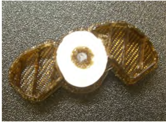
Figure 2-2 Cross-sectional view of the vascular model during the build process
