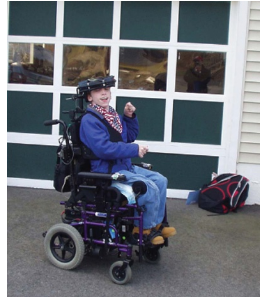
Head controlled wheel chair steering system for a boy unable to use a joystick
