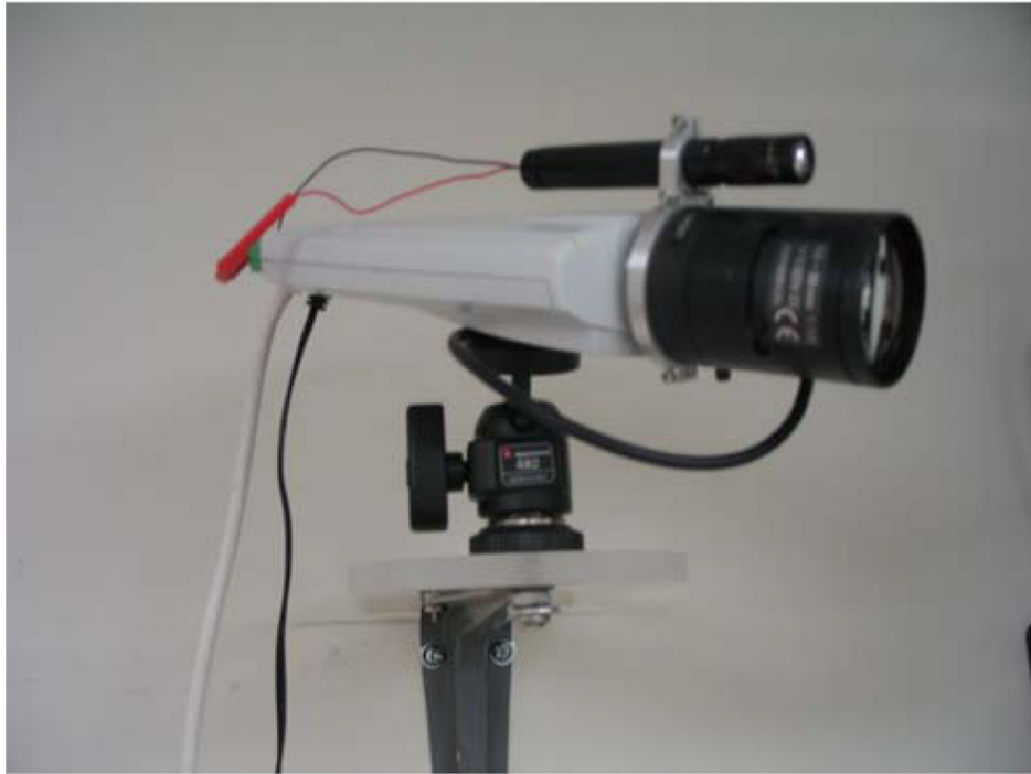
Figure 3. One of our Axis 211 cameras with LED on top which was powered via camera and controlled through Axis software API's . The camera is securely mounted on wall pointed in the desired direction with a Manfrotto tripod head.
