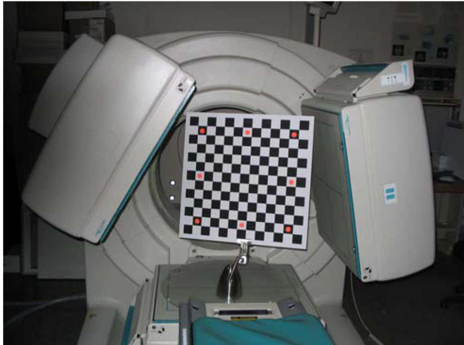
Figure 1. The planar calibration pattern that we fabricated supported with a weighted-flexible base in between the heads of our SPECT system.
