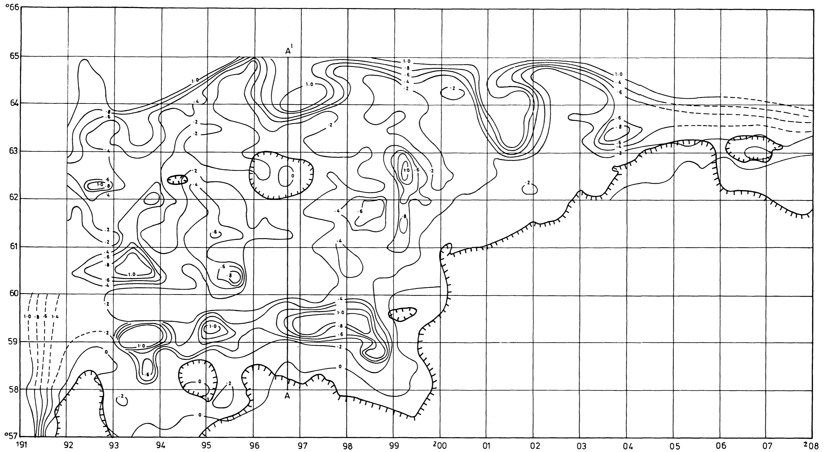
FIG. 5(c) ST. AUSTELL AREA - DEPTH OF GRANITE BELOW SEA LEVEL IN Km
