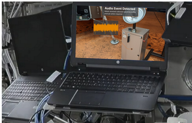
Figure 1: Integrated audio perception into the telerobotic system of Surface Avatar. The robot in the experimental area detected a sound event with an unknown spectral profile and requests manual action from an astronaut on board the International Space Station (ISS).
