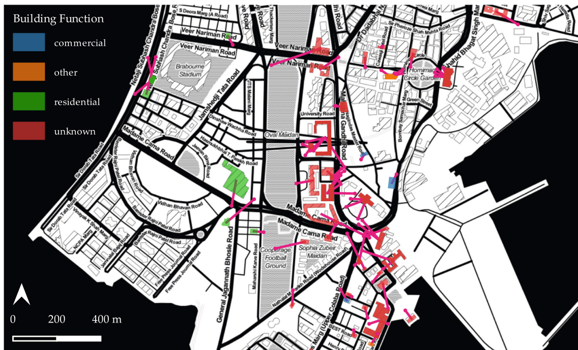
Fig. 8. Map of Flickr images in Mumbai spatially aligned with buildings. Magenta lines indicate the line of sight from an image toward a building. Buildings are colored based on their function as described in OpenStreetMap. (For interpretation of the references to colour in this figure legend, the reader is referred to the web version of this article.)
