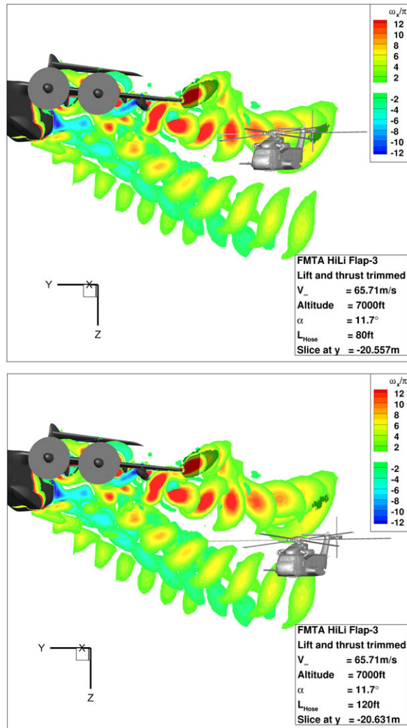
Figure 6. Helicopter’s pre-contact position in tanker wake flow for the 80ft (top) and 120ft hose (bottom).
