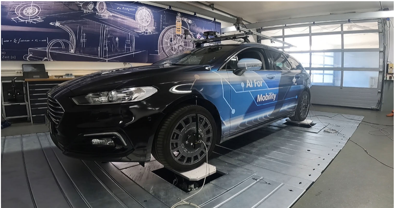
Figure 4. AFM experiments on a vertical dynamics test rig.
