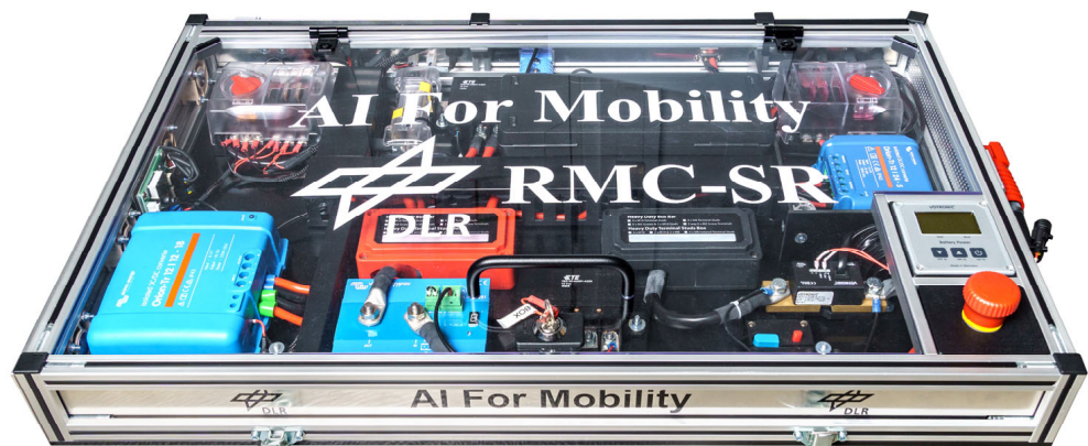
Figure 9. The E-Box with all electrical components necessary for the operation of all auxiliary equipment (sensors, actuators, computers, etc.).
