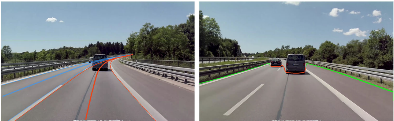
Figure 6. Application of state-of-the-art neural networks for path detection (left) and free space detection (right) on a highway.
