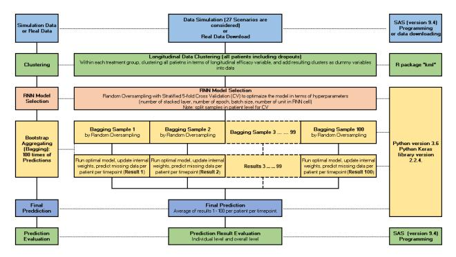
Figure 3. Diagram of Workflow– overall process for handling missing data in longitudinal continuous variable.
