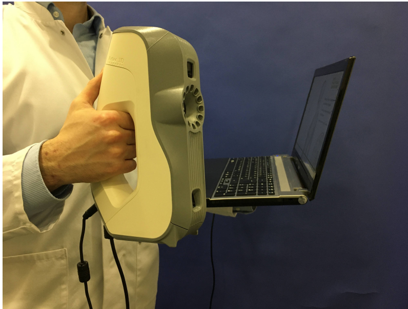
Abbildung 1.2: In Publikation 1 erprobter Artec Eva Strukturlicht 3D Scanner. Abbildung aus Koban, K.C. et al. Three-dimensional surface imaging in breast cancer: a new tool for clinical studies? Radiation Oncology ( https://doi.org/10.1186/s13014-020-01499-2 ) lizenziert unter Creative Commons Attribution 4.0 ( http://creativecommons.org/licenses/by/4.0/ ).
