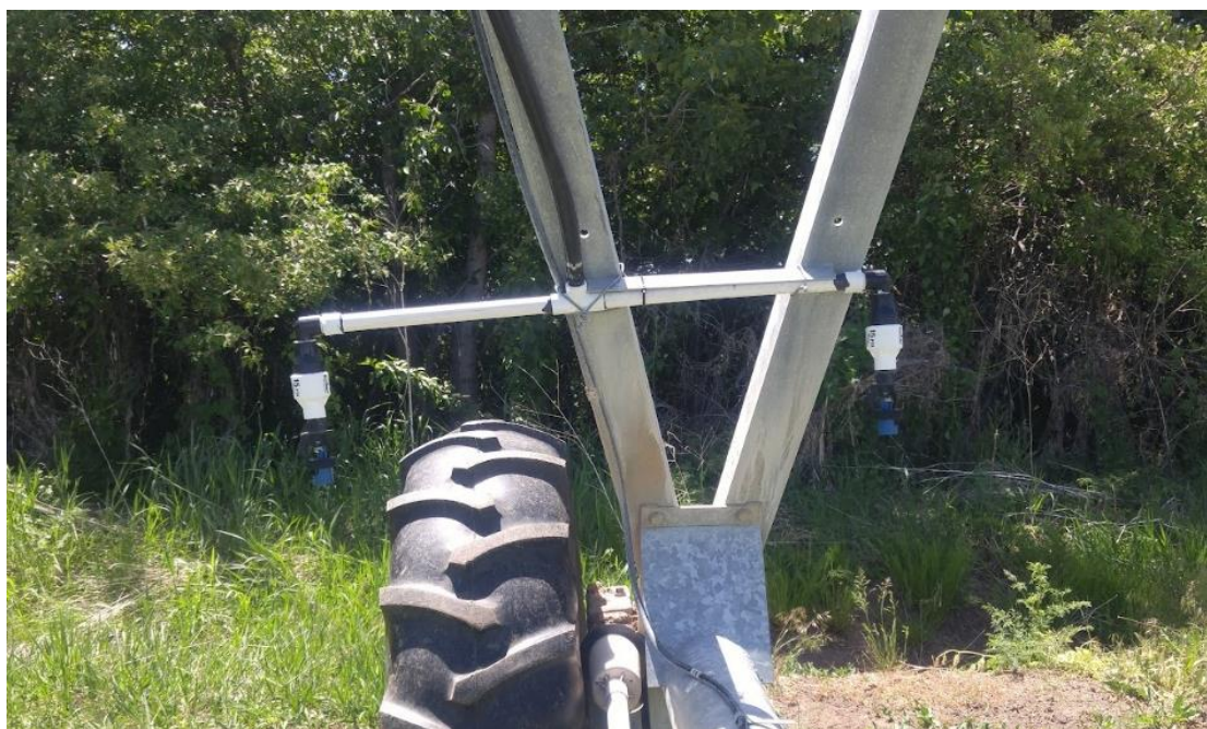
FIGURE 3.3 Two part circle sprinklers mounted to a PVC pipe manifold, attached to a pivot tower, as part of the double part circle method
