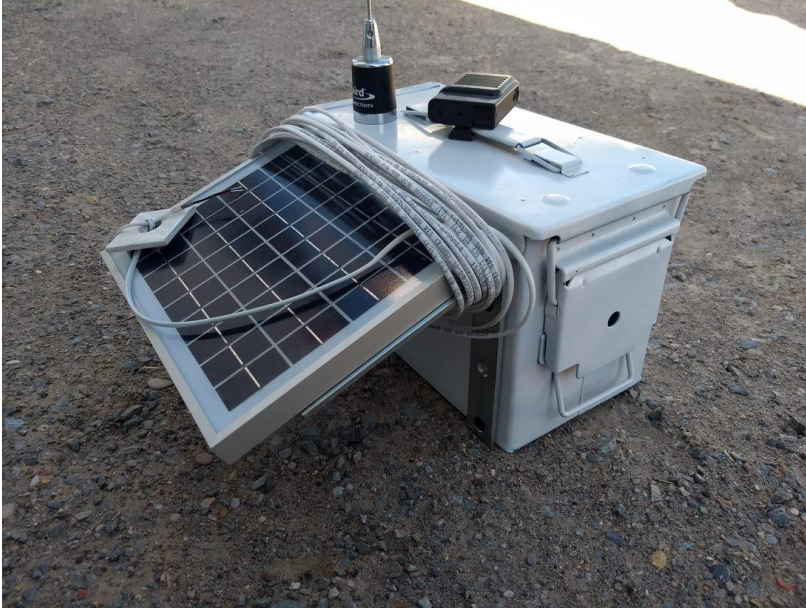
FIGURE 5.2 Irrigation advance sensor developed by Commercial Business Radio (Photo by Kalen Taylor)
