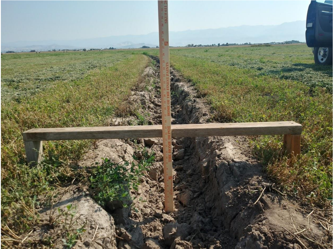
FIGURE 3.11 Track depths were measured from the bottom of the wheel track up to a 1 m long plank, which was suspended above the soil surface on two 0.15 m legs to avoid soil ridges alongside the wheel track.
