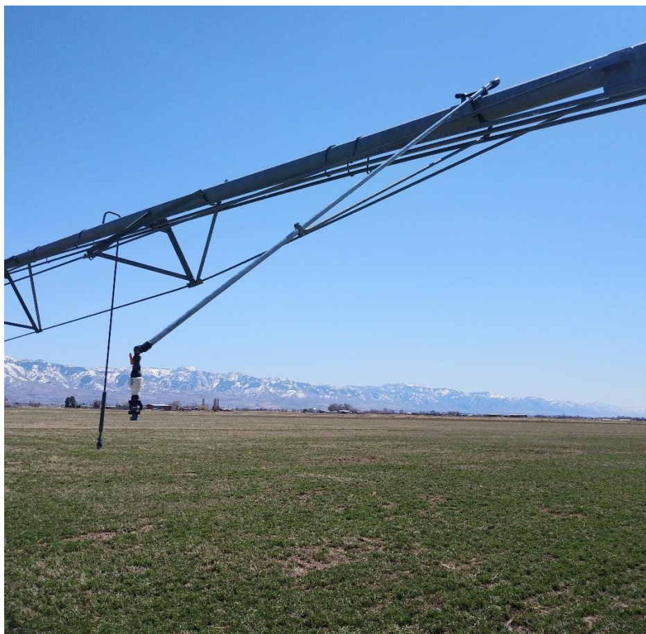
FIGURE 3.9 A single-boom attached to a pivot, intended to direct water behind the direction of travel
