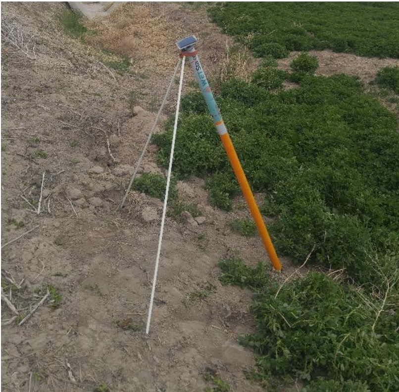
FIGURE 5.3 "Wet Stake" irrigation advance sensor developed by Prescott Farm Innovations
