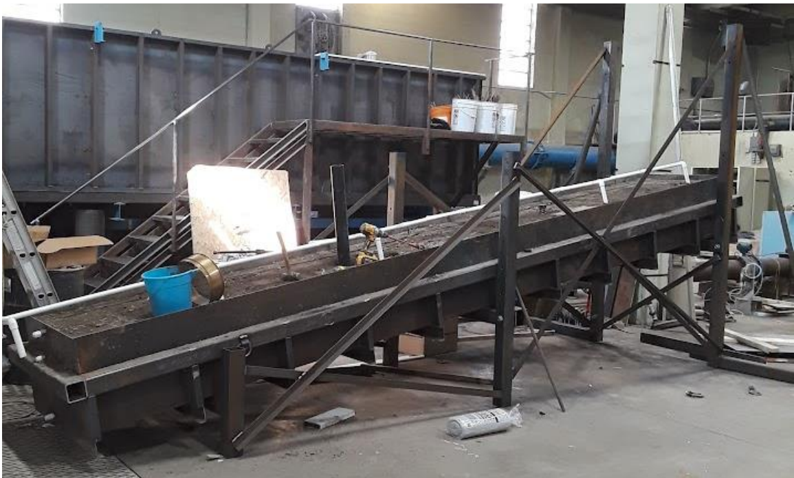
Fig. 9. Apparatus on support structure and installation of soil moisture sensor.
