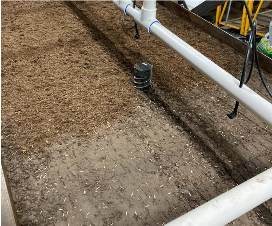
Fig. 12. Application of seed mix and peat moss.
