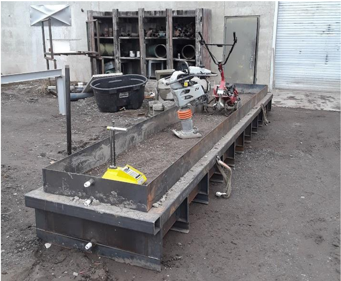
Fig. 8. Compaction and testing of material in apparatus.
