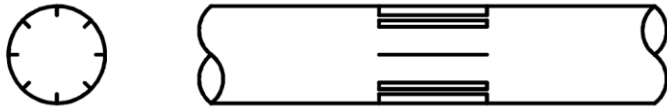
Figure 5. Depiction of Straightening Vanes in a Pipe: Cross-Section View (left) and Side Cutaway (right)
