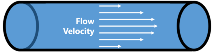
Figure 1. Drawing of Flow Velocity (Speed) in a Full-Flowing Pipe
