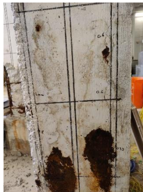
Figure 6-16. State of column L-15-Str after the accelerated corrosion program
