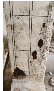
Figure 6-16. State of column L-15-Str after the accelerated corrosion program
