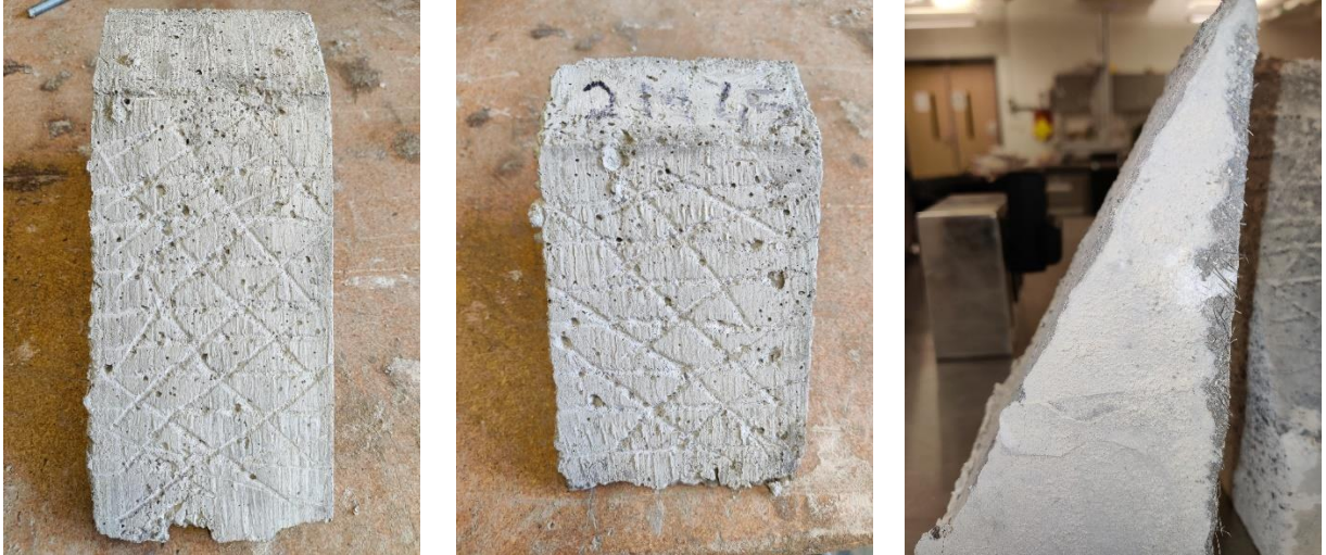
Figure 8-2. Interface surface prior to UHPC addition
