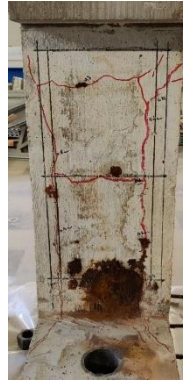
Figure 6-14. State of column S-20-Cor after the accelerated corrosion program
