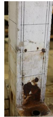
Figure 6-18. State of column L-20-Str after the accelerated corrosion program
