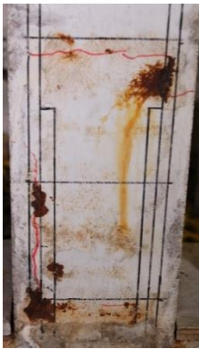
Figure 6-10. State of column L-20-Cor after the accelerated corrosion program
