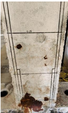
Figure 6-16. State of column L-15-Str after the accelerated corrosion program
