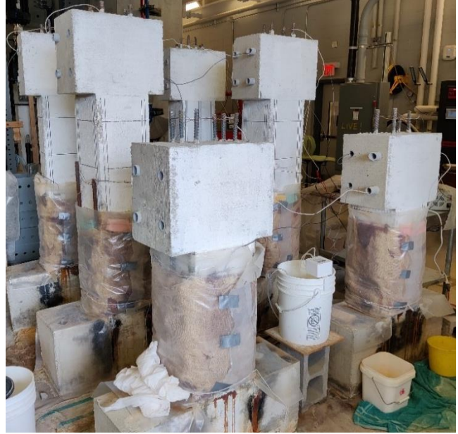
Figure 6-6. Photos from the accelerated corrosion program. Short column with cathode bars shown before covering with second layer of burlap and a plastic sheet (left). All columns are shown during a wetting cycle (right).
