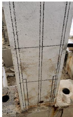
Figure 6-16. State of column L-15-Str after the accelerated corrosion program
