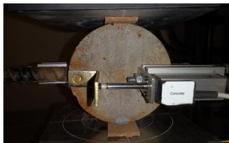
Figure 4-2. Specimen Pre-Cracking Splitting Setup and Instrumentation. Rust stains were caused by oxidation of steel fibers during the curing period and not from accelerated corrosion which followed this stage.
