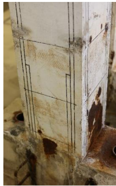
Figure 6-18. State of column L-20-Str after the accelerated corrosion program
