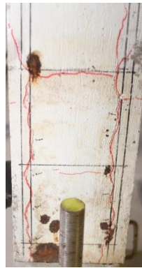
Figure 6-10. State of column L-20-Cor after the accelerated corrosion program
