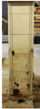
Figure 6-18. State of column L-20-Str after the accelerated corrosion program
