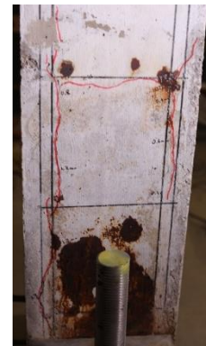
Figure 6-10. State of column L-20-Cor after the accelerated corrosion program
