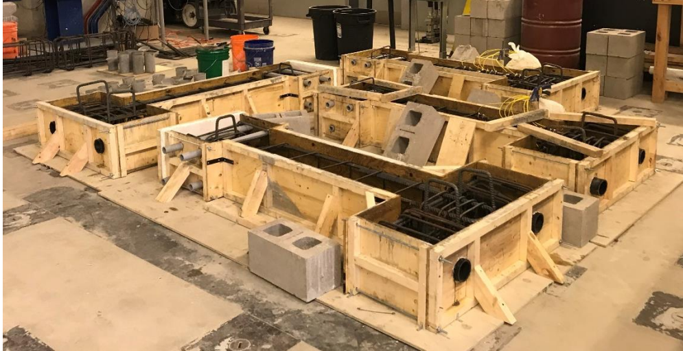
Figure 6-4. Specimens ready for casting
