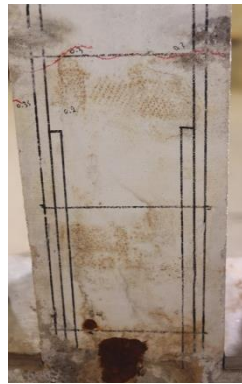
Figure 6-10. State of column L-20-Cor after the accelerated corrosion program
