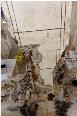
Figure 6-18. State of column L-20-Str after the accelerated corrosion program
