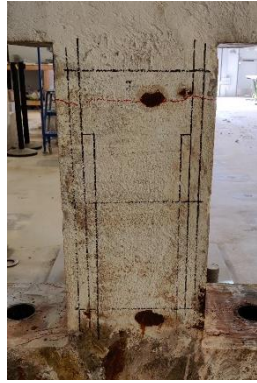
Figure 6-14. State of column S-20-Cor after the accelerated corrosion program
