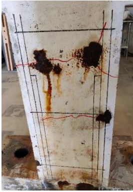
Figure 6-14. State of column S-20-Cor after the accelerated corrosion program
