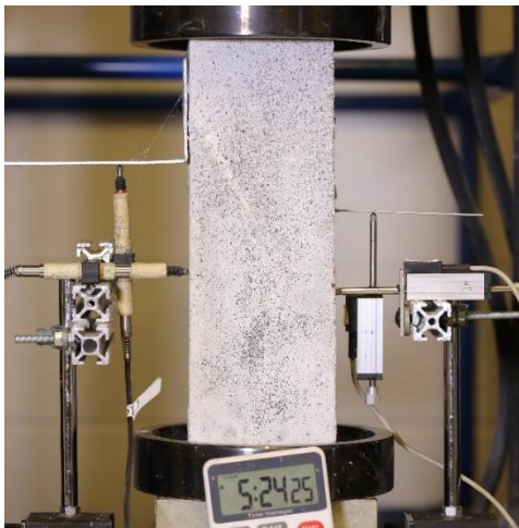
a) Slanted Shear Test
