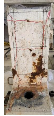
Figure 6-14. State of column S-20-Cor after the accelerated corrosion program
