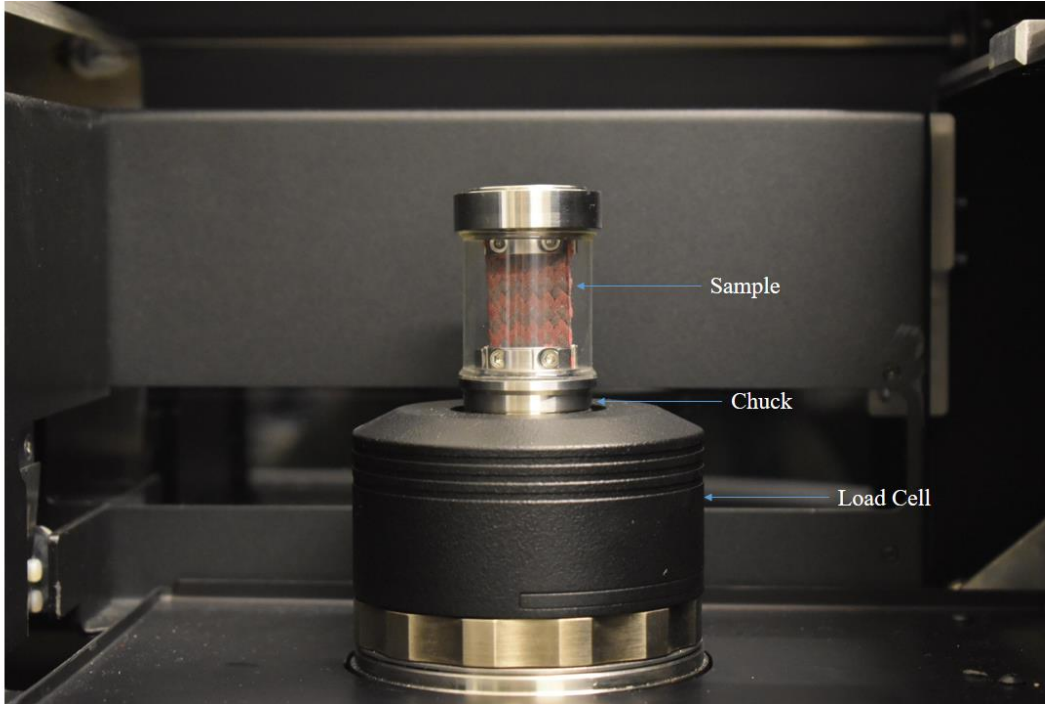
Figure 4-3: Setup View of Material Testing Stage inside Micro-CT. The sample holder holds the sample, chuck holds the sample holder & connects to the load cell and load cell is used to apply forces in tension or compression.
