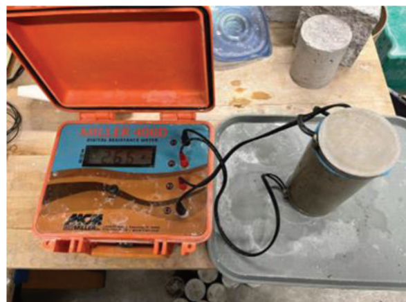
Figure 6.1 The setup of resistivity measurement.
