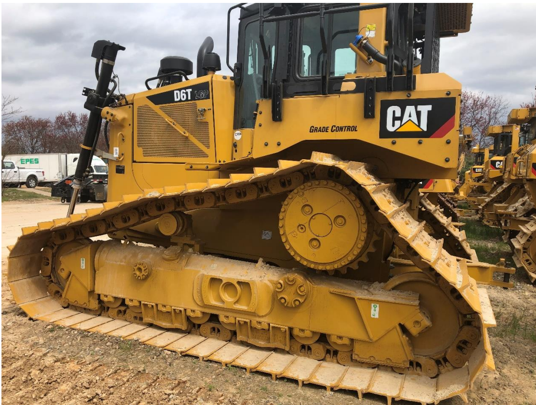
Figure 1. Heavy Construction Equipment Undercarriage System
