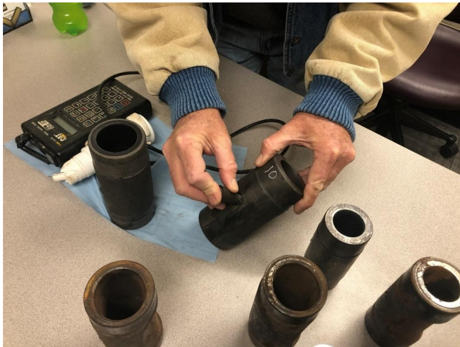
Figure 30. Gage R&R Measurement Process
