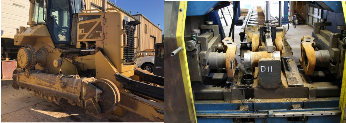
Figure 6. Bushing turn Maintenance of Rotating the Track Bushing
