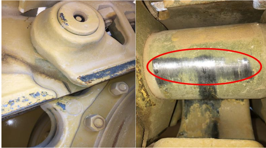
Figure 4. Sprocket and Track Bushing Wear Surfaces
