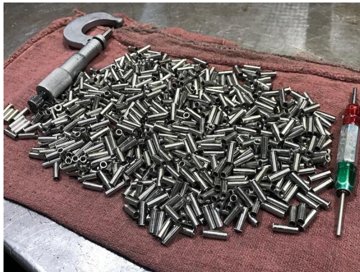
Figure B2: Fasteners being sorted due to a defect found during machining.
