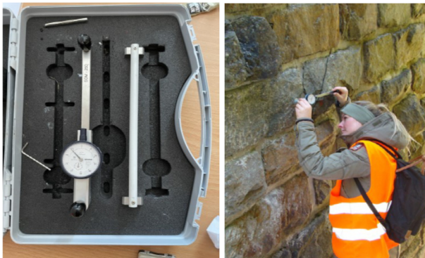
Fig. 3: Deformeter SDM 250/10 and a practical example of measuring the width of the monitored crack.
