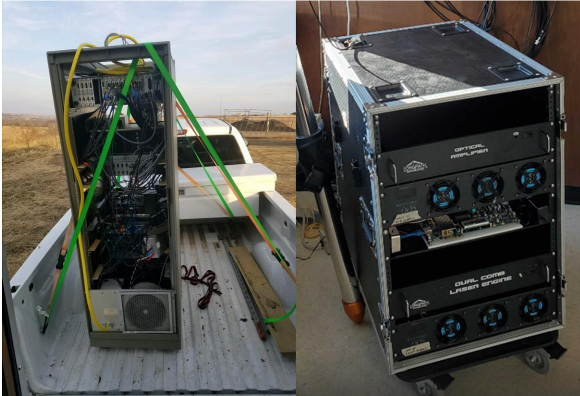
Figure 2.4 The DCS rack from our first experiment, discussed further in Chapter 3, is pictured on the left. The rack was compact enough to be moved but was far too heavy to escape the use of a forklift. On the right, the newly packaged system is far more compact, integrated as a full system, and light enough to be lifted by two people. Photo credits to Eduardo Santos and Brian Washburn.
