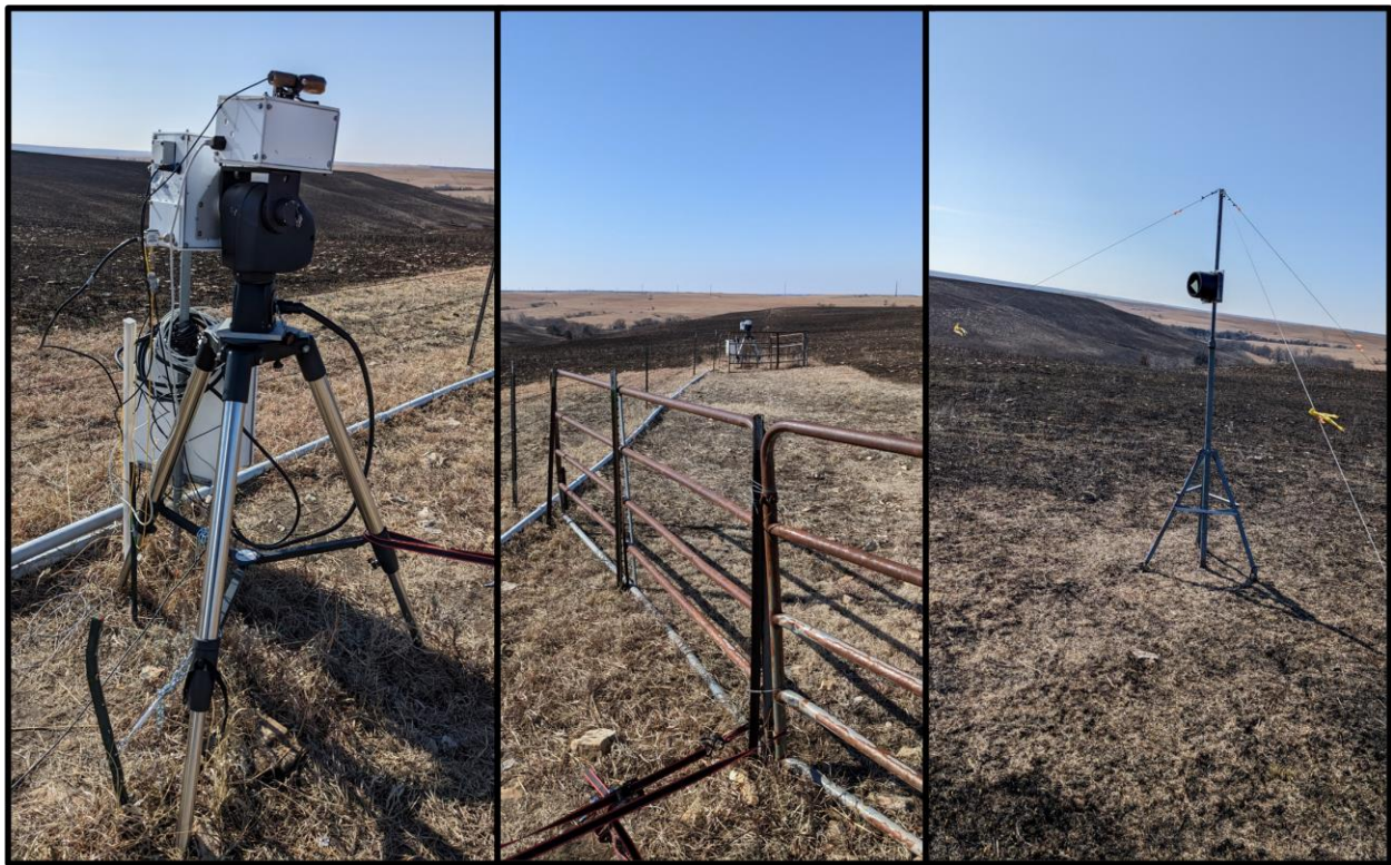
Figure 4.6 Left: North transceiver; note the box for electronics staked beside the tripod. Updated transceivers allocate protective housing for the camera, while having a modified flashlight mounted up top for flashing in nighttime alignments. Center: From North transceiver, an image of the South transceiver. Note the cattle pen gating used to protect transceivers from future animals, as well as conduit against the fence line. Right: Retro 1 on its stabilized tripod.
