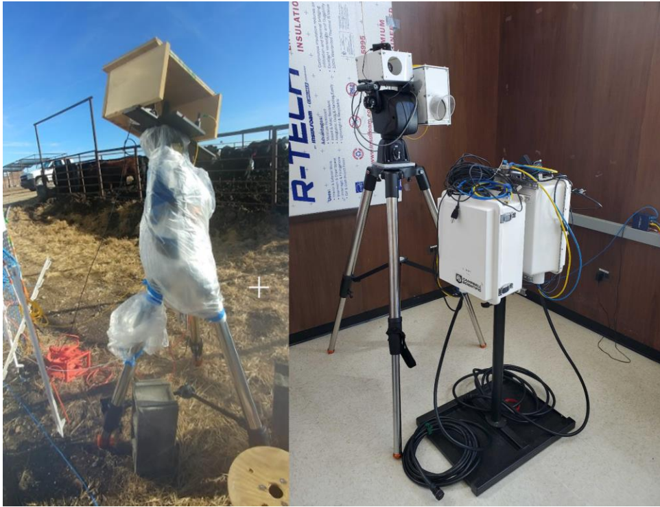
Figure 4.2 To the left, the transceiver used during the feedlot can be seen. While this was functional, it was not ideal, and left room for improvements in harsh weather conditions. To the right, the newly improved transceiver is pictured. These protective boxes shield optics and the camera from the elements. The accompanying boxes keep equipment off of the ground and protected from most rodents and insects. Photo credit courtesy of Brian Washburn.
