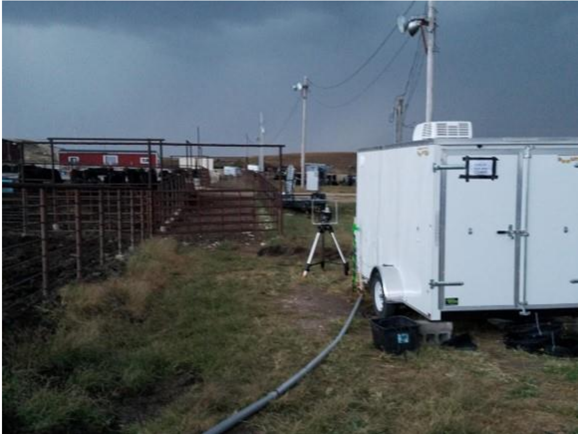
Figure 2.5 A view of the Agrocombs trailer parked on-site for our first measurement, discussed further in Chapter 3. The trailer houses most electronics and computers related to the Agrocombs system and our comparative system, the CRDS. The trailer’s temperature control is adequate to keep the combs stable, while access into the trailer is granted through portholes. Photo credit to Brian Washburn.
