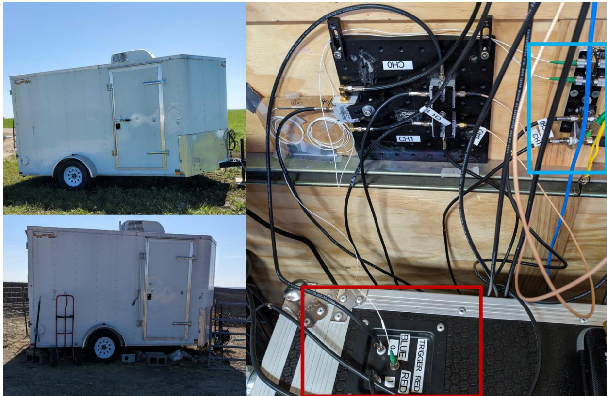
Figure 4.4 In the top left, our new beginning on the Rannels Ranch as we park the trailer in the pasture. In the bottom left, one can see the trailer in its current state, with the surrounding pasture recently having been through a controlled burn. To the right, the top of the DCS rack (seen in full in Figure 2.4). The red area shows the ports added for fiber and DAQ connections. In the light blue area, one can see the wall-mounted fiber and rf cables that allow us to strain relieve these connections, as well as easily access them.
