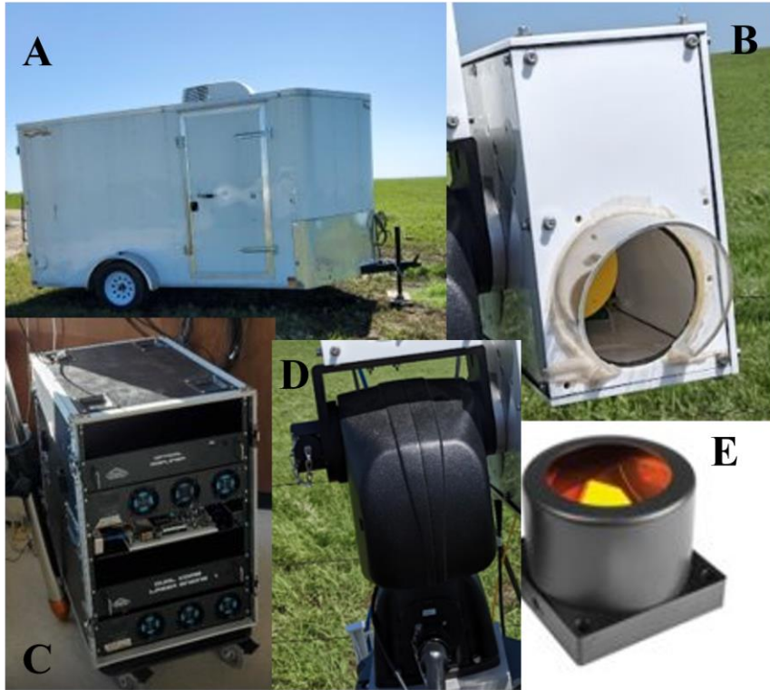
Figure 2.3 Images of main components of the Agrocombs system. A) Our mobile lab that houses the DCS system and additional tools. B) Optical transceiver, designed to transmit light across beam path and receive returning light to a photodiode. C) DCS rack, housed in our mobile lab. The rack is compacted to contain a fiber-based laser system and a rack-mounted computer. D) Gimbal for mounting transceivers, capable of movement for optical alignment. E) Retroreflector used to reflect light back into transceiver, mounted on the opposite side of the beam path from the transceiver.
