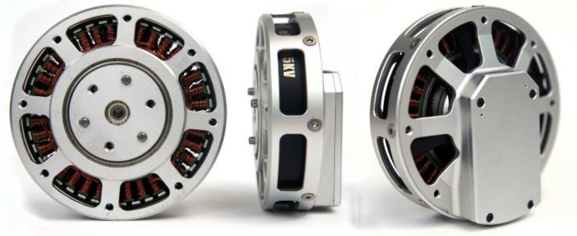
Figure 2: MIT Cheetah III Actuator Designed by Ben Katz [7]
