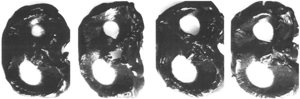
Figure 4.12: Photographs of the boundaries of the contact area without the menisci as reported by Fukubayashi and Kurosawa [62].
