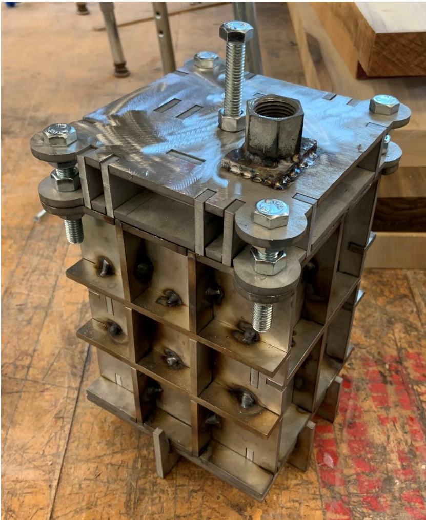
fig. 5: Complete plastic brick mold assembled
