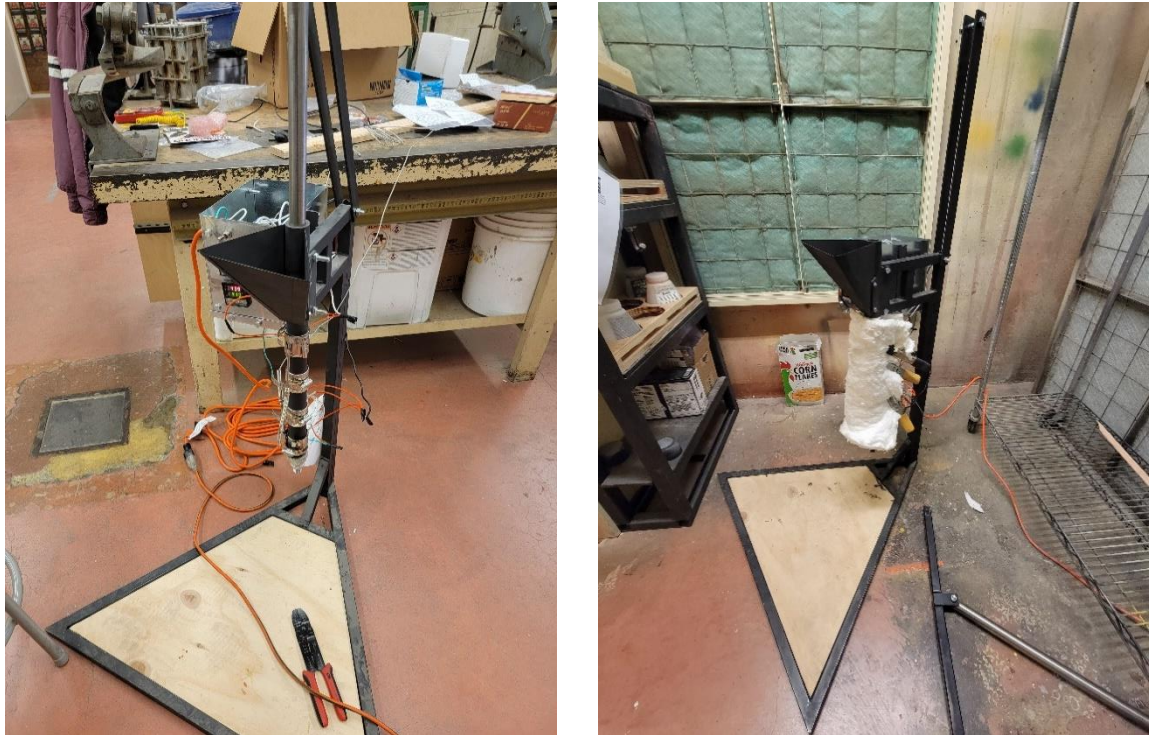
fig 18: (L-R) Injector's original layout; Injector after insulation was added.
