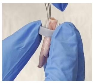
Figure 25: First step of assembly: Pulling blood vessel through middle hole.
