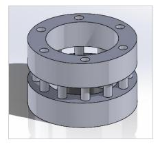
Figure 16: Assembly of Coupler Rings
