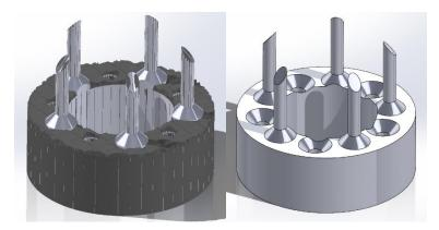
Figure 21: Image of Model A Mesh showing Knurled Surface Texture
