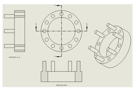
Figure 18: Drawing of Individual Pins
