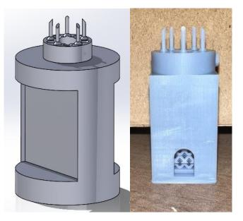
Figure 30: Connection Force Testing Fixture: Solid works first sketch (left), Model used in Testing (right)
