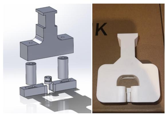
Figure 31: Vessel Grip Test Fixture: Solid works first sketch (left), Fixture used in Testing (right)
