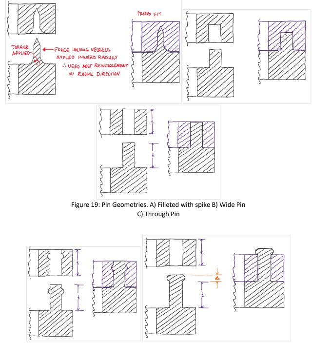
Figure 20: Pin Geometries. D) Male Female Interlocking E) Through Male
