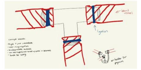
Figure 14: Rigid T Joint Prosthetic with Ligations
