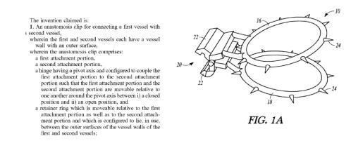
Figure 6: US-11259809-B2 March 1st, 2022: Blood vessel connectors and methods for blood vessel connection
