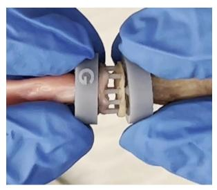
Figure 28: Fourth step of assembly: Coupler arrangement before mating.
