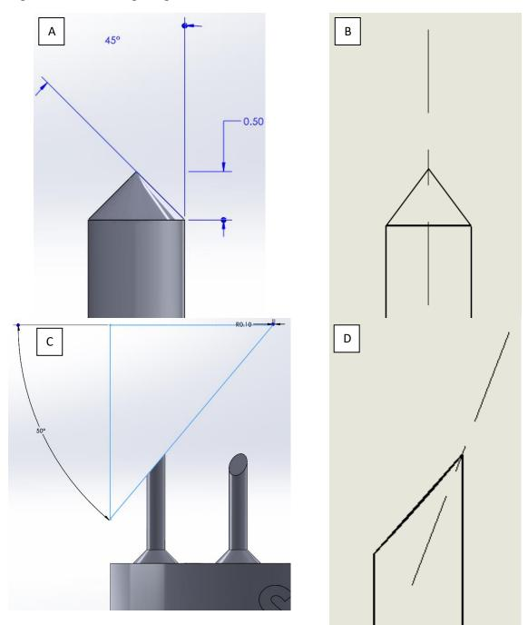
Figure 23: Spike Design. A) Old spike geometry. B) Old Angle of point apex. C) Latest spike geometry. D) Latest Angle of point apex.
