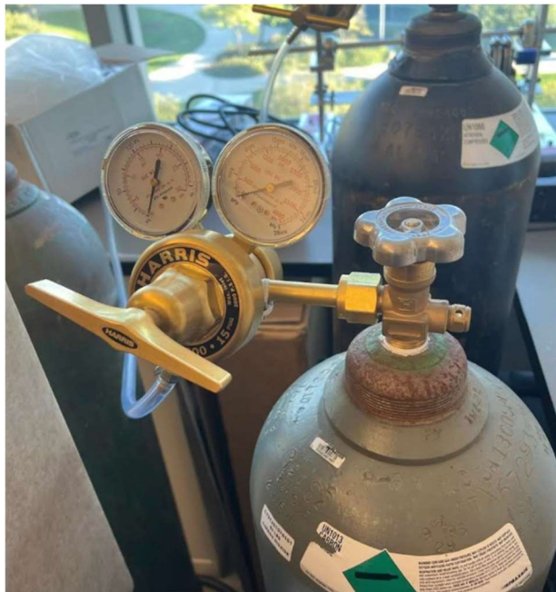
Figure 11. Air pressure regulator assembled onto the CO2 gas tank
