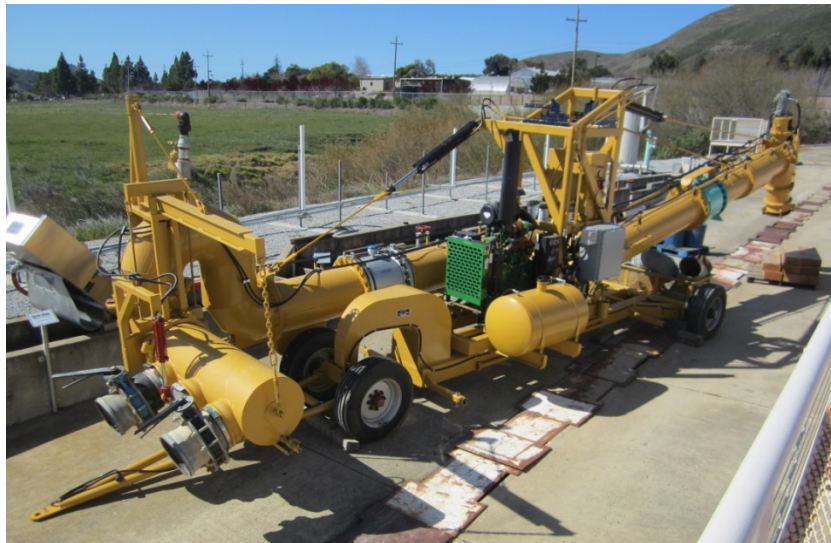
Figure 3. Pumping system for IID jack gate characterization
