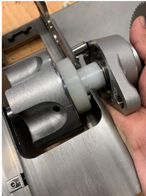
Figure 11: Shaft being lowered into place
