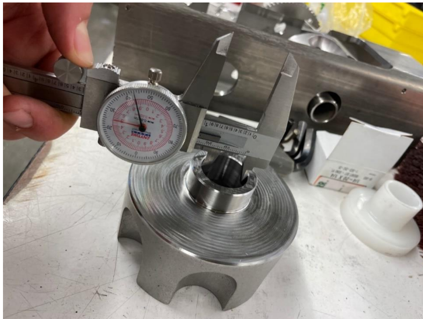
Figure 9. The finished wheel has too large of a hole for the shaft to pass through.
