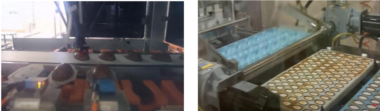
Figure 1. Kinder Joy Egg Assembly Operation Moving Rounded Shells Similar to CoolBeans
