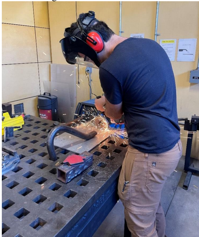
Figure 17. Adin using the angle grinder on the base plate to cut out the slot
