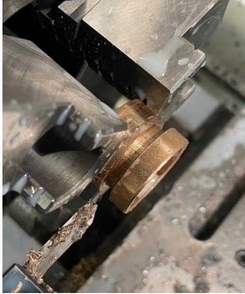
Figure 13. A parting tool us used on a lathe to cut a ¼ inch slice off of a bronze bushing.
