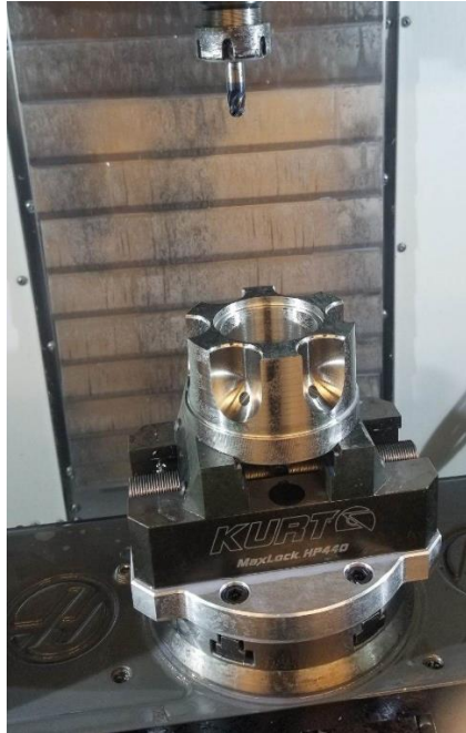
Figure 8. Wheel Fixtured in CNC mill
