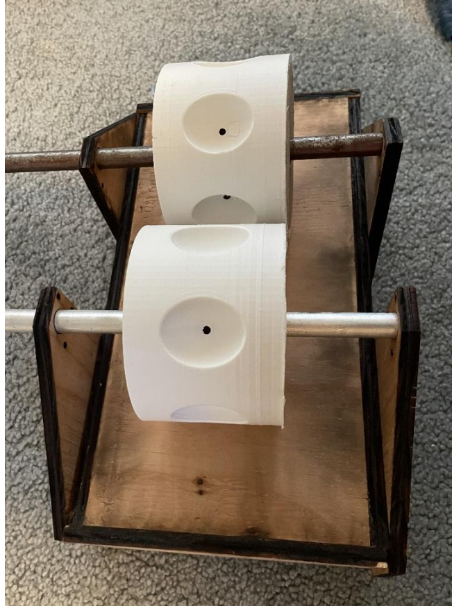
Figure 9: Laser Cut and 3D Printed Concept Prototype.
