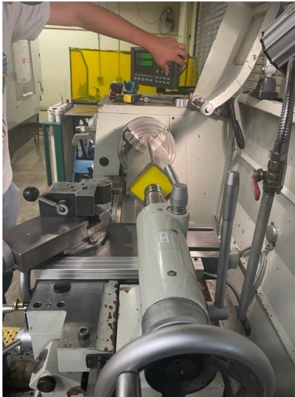
Figure 11. The square tube having its ends faced on the lathe before being fixtured in CNC mill
