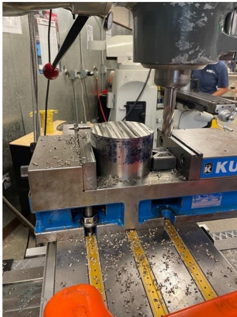
Figure 7. The round stock is face milled on manual mill to be fixtured in CNC mill
