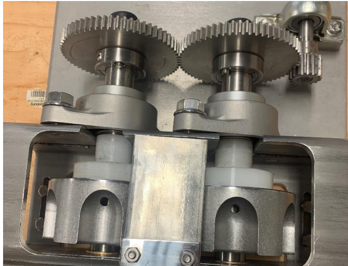
Figure 1: Shaft Assemblies in Place With all Components Installed
