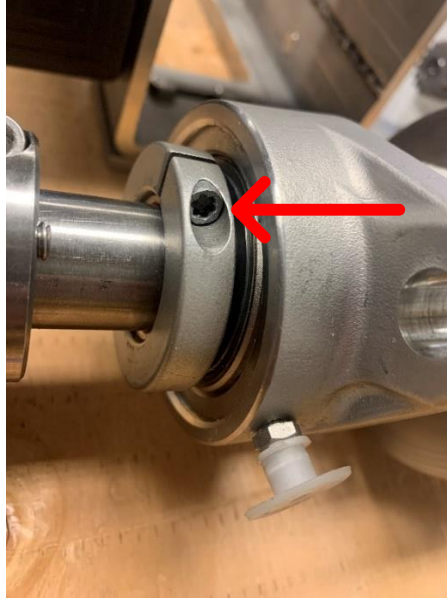
Figure 7: Bolt that needs to be loosened to remove bearing from shaft.
