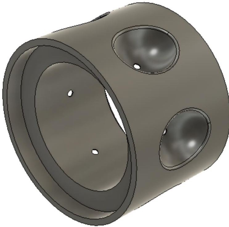
Figure 11: CAD model of vacuum wheel design.
