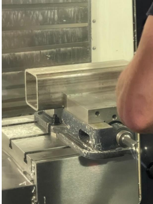
Figure 10. The square tube fixtured in the CNC mill
