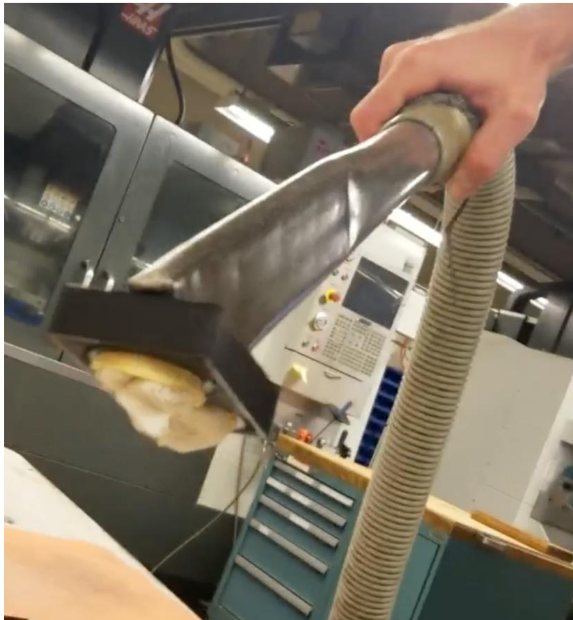
Figure 13: Vacuum Retention Test
