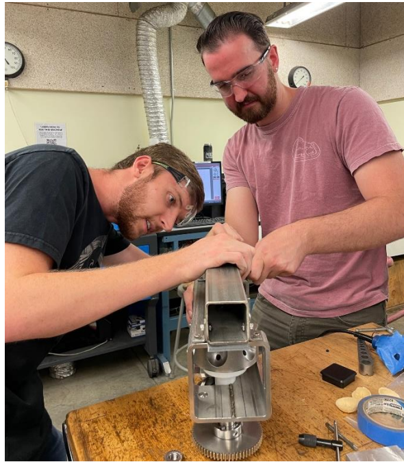
Figure 5. Assembly of vacuum tube with prototype frame
