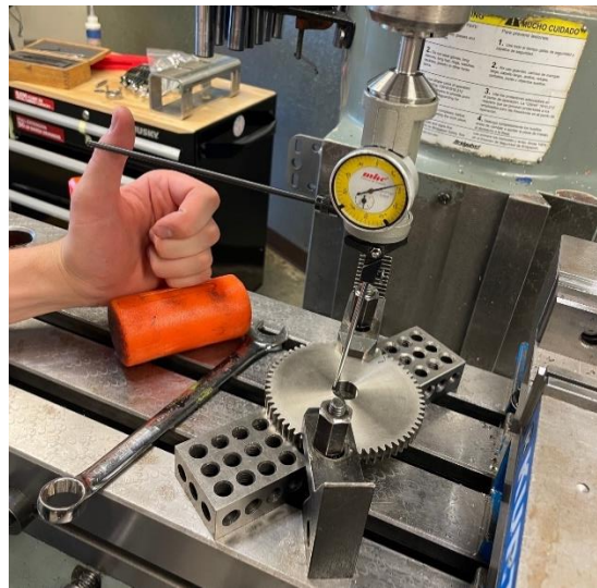
Figure 4. Gear modification fixturing and coaxial alignment with mill spindle
