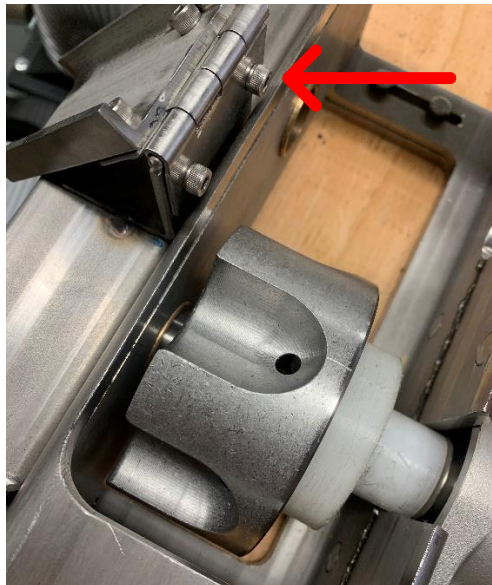
Figure 2: Image showing the finger guard lifted out of the way
