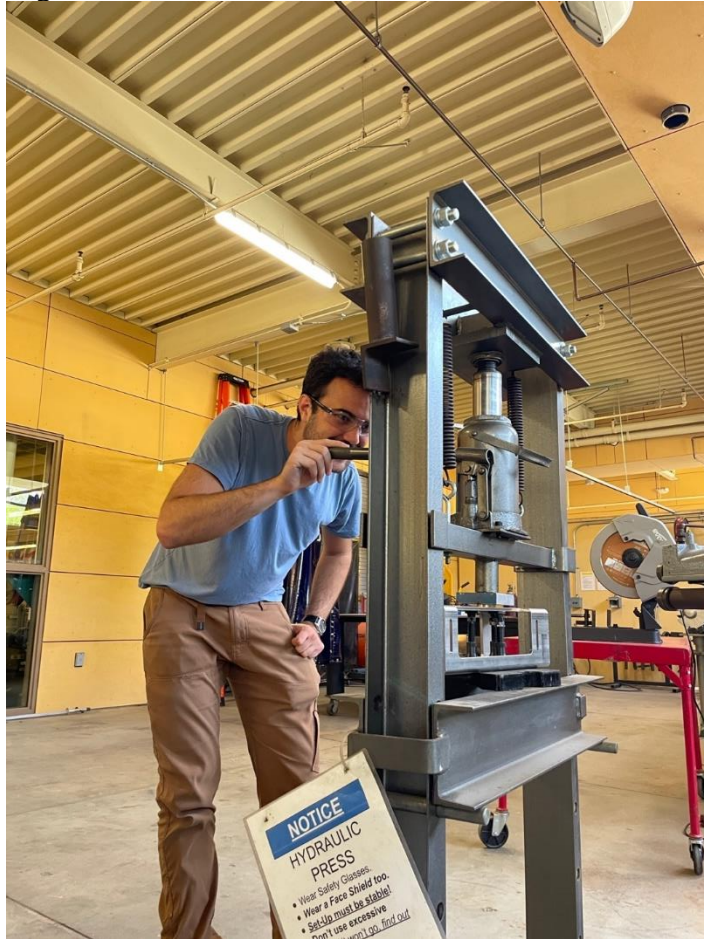
Figure 14. Press fitting the bushings into the square tube with hydraulic press. Black machinist screws keep the square tube from deflecting.
