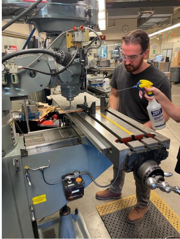
Figure 16. Milling the under-wheel section of the base plate
