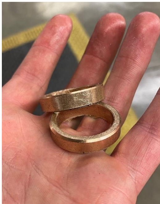
Figure 12. Bronze bushings cut to size and chamfered
