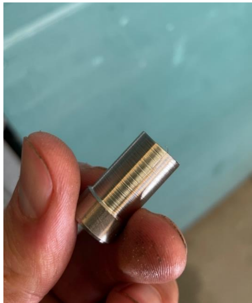
Figure 15. A finished unthreaded pin. The threaded pin is slightly longer.
