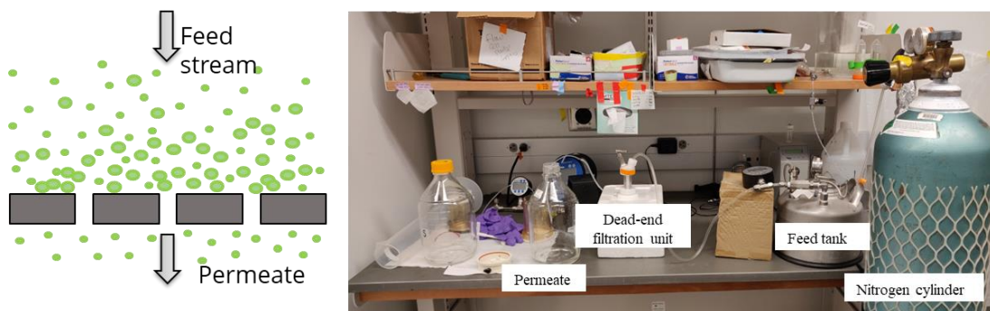
Figure 4.2: a) Schematic of working principle of dead end filtration system
