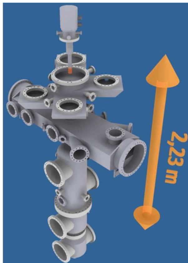
Fig. 84. Layout of the new target inlet chamber design with the existing interaction chamber and target dump system for the ESR in Darmstadt.
