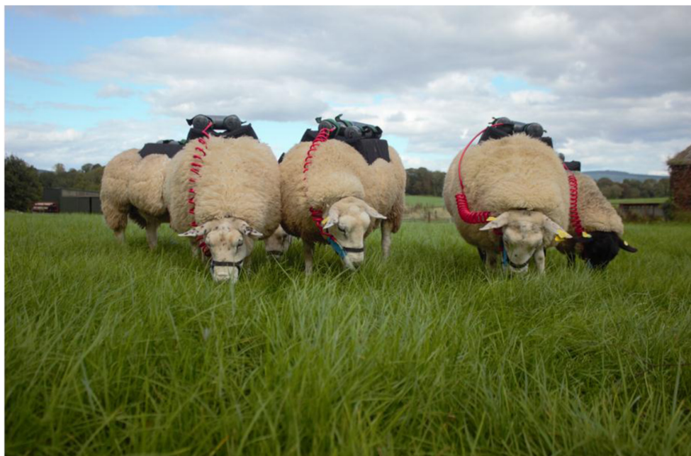
Image 2. SF 6 equipment on grazing sheep, Teagasc, Athenry, Co. Galway.
