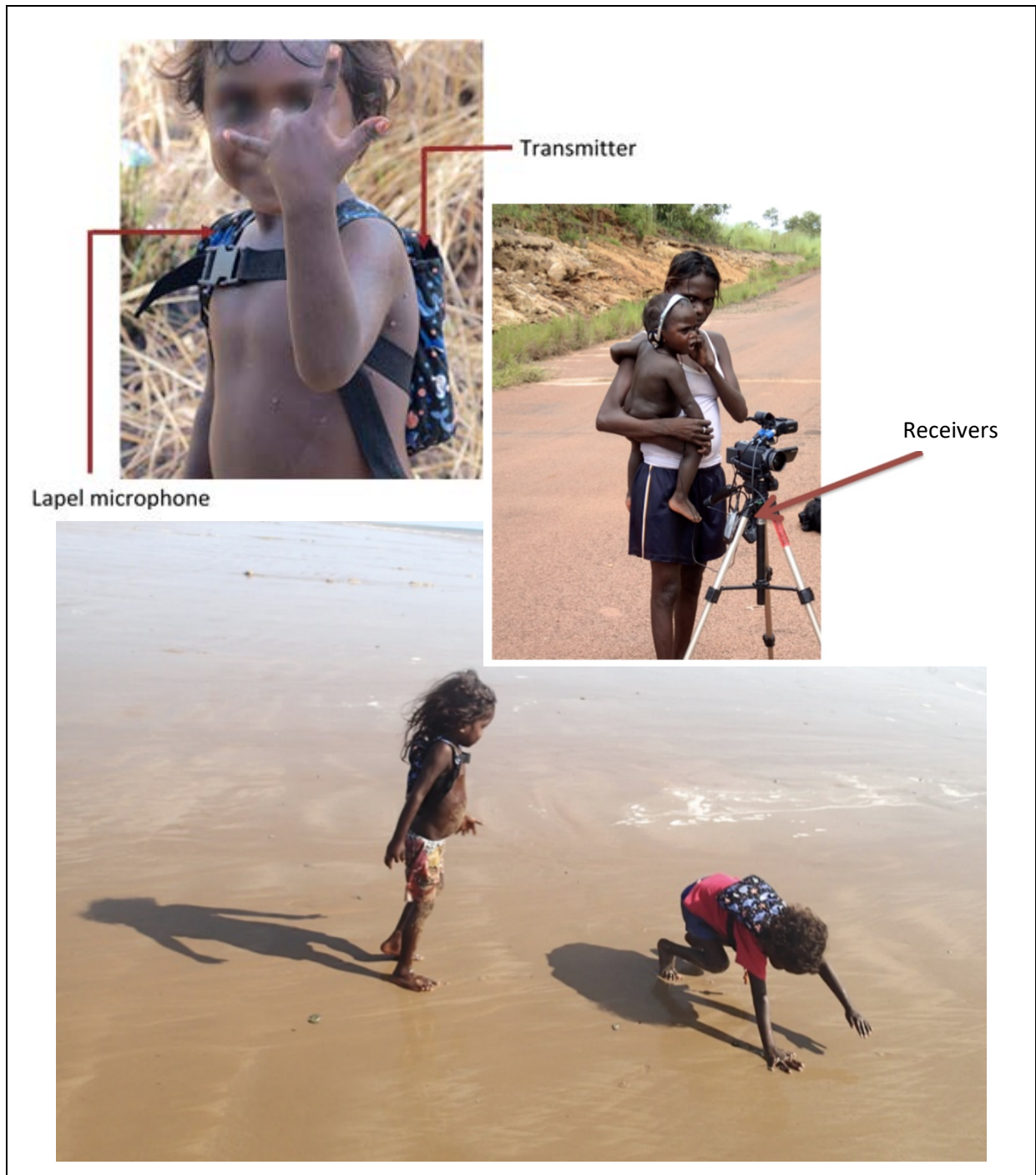
Figure 1. Example of recording setup (photos: Lucinda Davidson), showing the location of the transmitter and hidden lapel microphone in the child's backpack, and the receiver plugged into the camera. Children are free to run about while wearing the backpacks.
