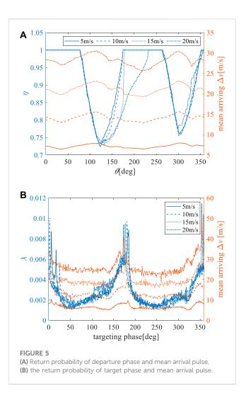
phases in which almost 100% can return DRO are mainly distributed in two regions:  $[0^{\circ}, 80^{\circ}]$  and  $[230^{\circ}, 260^{\circ}]$ , and the velocity difference of the corresponding return point was relatively small. When the phase in these regions is selected as the phasing start point (initial pulse application point), the phasing orbit has high fault tolerance for the pulse direction, high safety, and a small escape risk.
