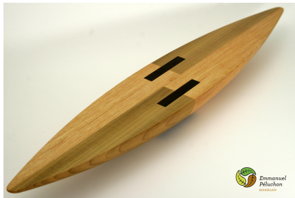
Figure 1.4: A rattleback [5]. When spun the rattleback wobbles to a halt before reversing direction.
