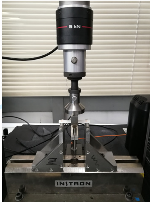
Figure A.1. Universal test machine with the tested beam sample for flexural modulus testing.
