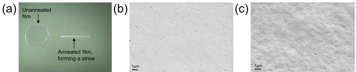
Figure 1. (a) Photo of SC-PLA film and straw. (b) SEM image of unannealed SC-PLA film and (c) SEM image of annealed SC-PLA straw.
