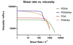
Fig. 3. Rheology of PGA, PDGA and hexanediol modifications.
