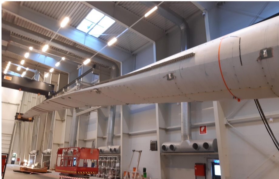
Figure 1. Wind turbine blade mounted on a test stand at Siemens Gamesa Blade Test Center in Aalborg, Denmark.
