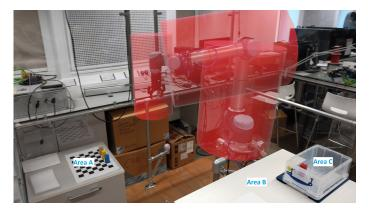
Figure 1: The robot arm picks up a wooden block from area A and moves it to area B, the middle of the table. The user then picks up the block from B and places it in the plastic container (area C).
