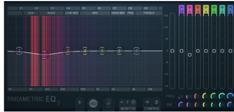
a Sub EQ curve with ‘dip’ around 100 Hz
