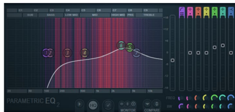
b ‘Scooped’ bass buss EQ curve with roll-off around 250 Hz
